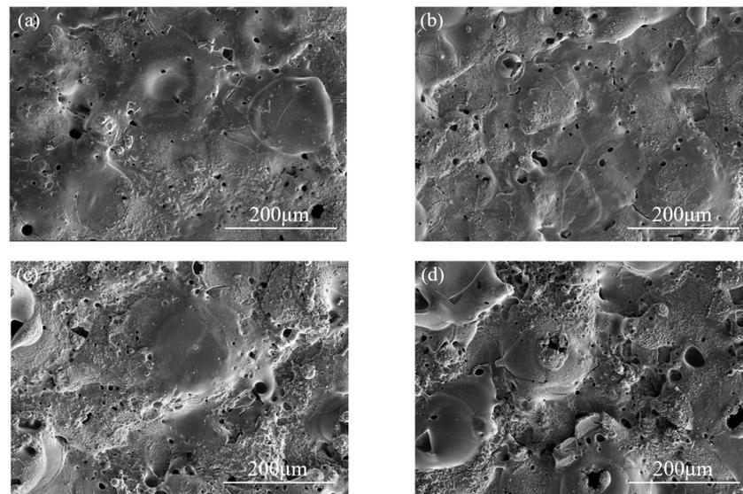
**Figure 3.** Surface topographies of the coatings after different high-temperature exposure times: (a) following 0 h of high temperature, (b) following 48 h of high temperature, (c) following 144 h of high temperature, and (d) following 288 h of high temperature.
