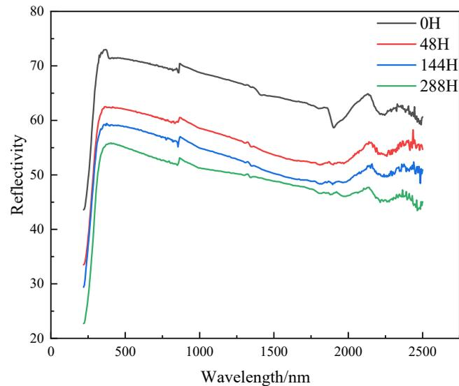
**Figure 1.** Reflectance curves of the coating after different holding times.
