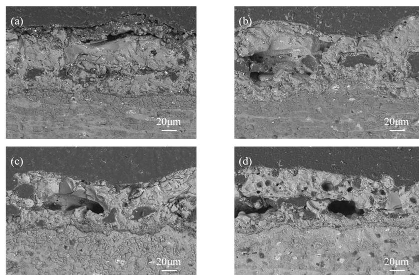
**Figure 4.** Cross-sectional topography of the coating after different high-temperature exposure times: (a) following 0 h of high temperature, (b) following 48 h of high temperature, (c) following 144 h of high temperature, and (d) following 288 h of high temperature.
