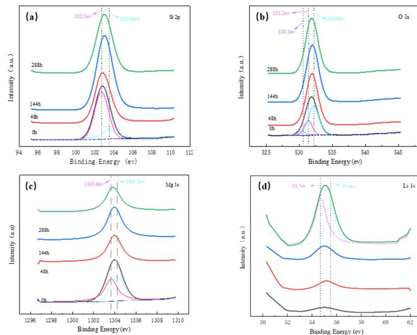
**Figure 5.** XPS spectra of the coating after different high-temperature exposure times: (a) Si 2p, (b) O 1s, (c) Mg 1s, and (d) Li 1s.
