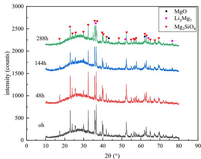
**Figure 2.** XRD spectra of coatings after different times at 200 °C.
