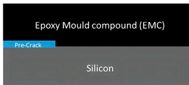
**Figure 1.** Schematic representation of the tested specimens.
