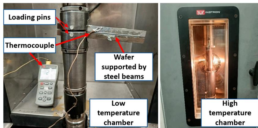
**Figure 4.** Testing procedure under low and high temperatures.
