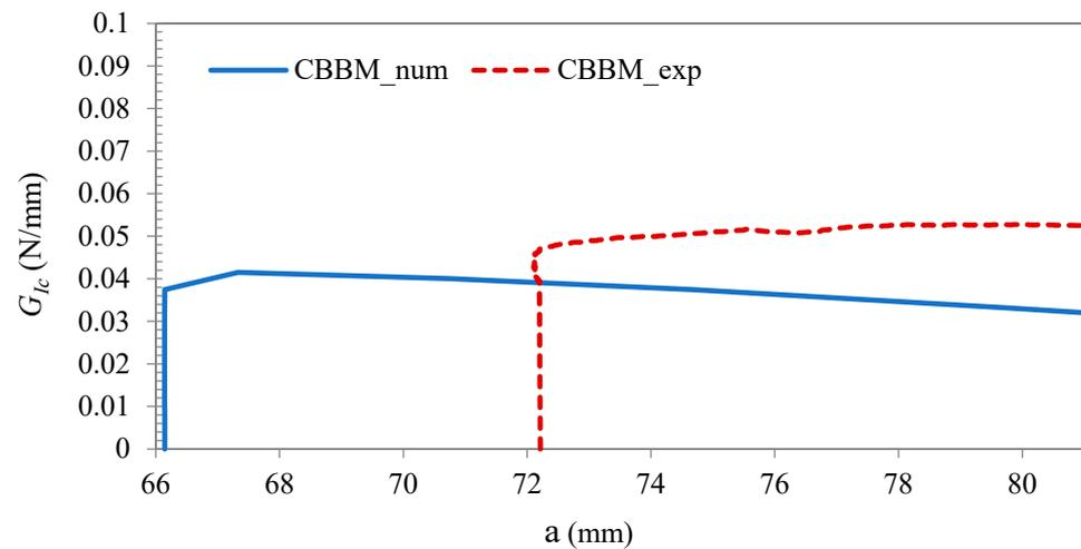
**Figure 12.** Comparison of numerical and experimental R-curves for the EMC-Si interface (Room temperature).
