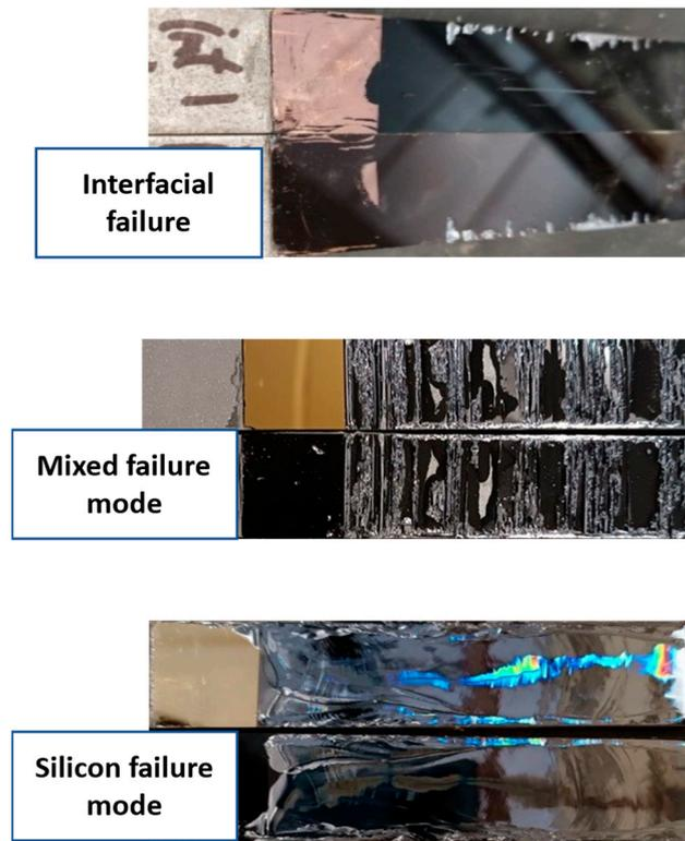
**Figure 9.** Different types of failure modes in wafers.
