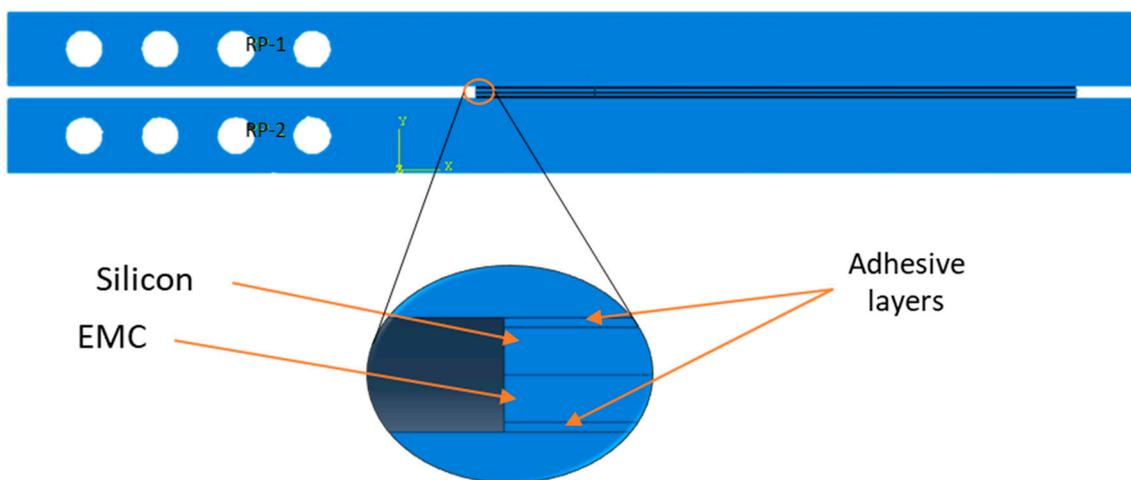
**Figure 6.** DCB assembly and different parts (wafer).
