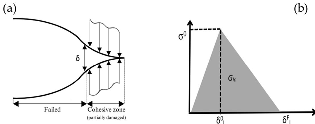
**Figure 5.** (a) CZM visual approach and (b) CZM traction separation curve.
