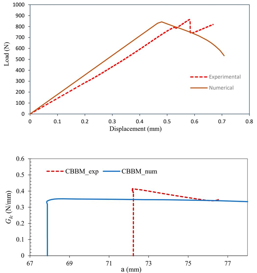
**Figure 15.** Comparison of numerical and experimental load–displacement and R-curves at high temperature (100 °C).
