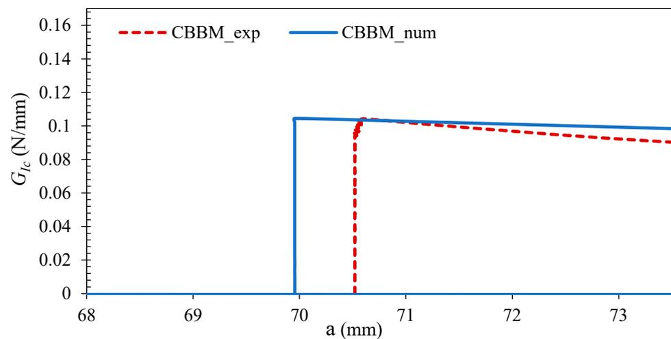
**Figure 14.** Comparison of numerical and experimental R-curves for the EMC-Si interface (low temperature).
