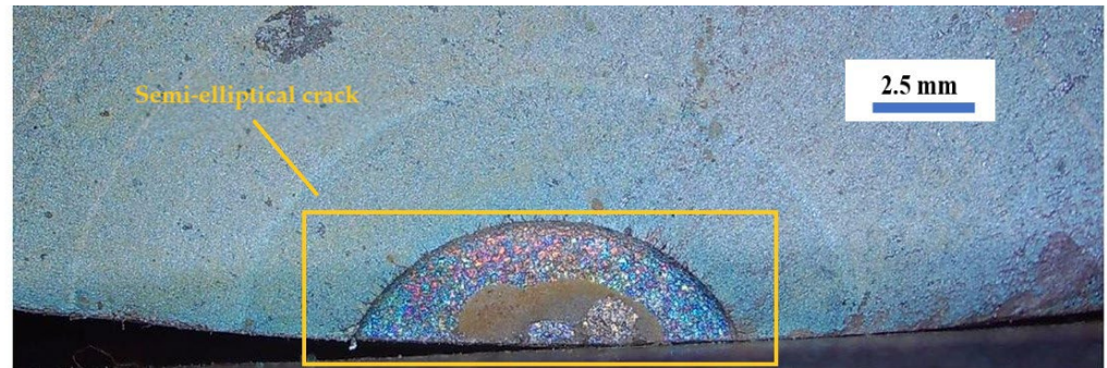
Figure 36. Semi-elliptical crack in the surface of a pipe [76].
