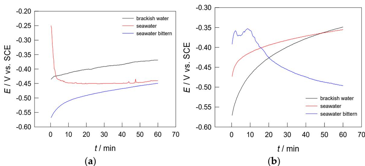
**Figure 1.** Open circuit potential measurements in brackish water, seawater, and seawater bittern for Ti (a) and Ti6Al4V alloy (b).
