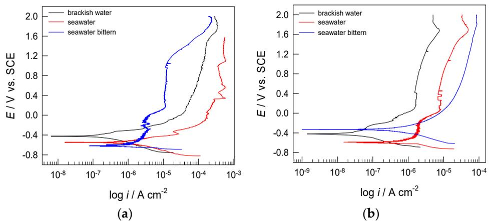
**Figure 3.** Potentiodynamic potential measurements in brackish water, seawater, and seawater bittern for Ti (a) and Ti6Al4V alloy (b).
