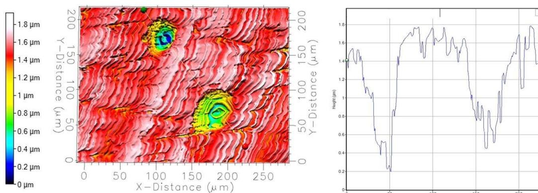
**Figure 11.** Three-dimensional appearance of corrosion pits and line profile measurement for Ti6Al4V electrode after potentiodynamic polarization measurements in seawater bittern.
