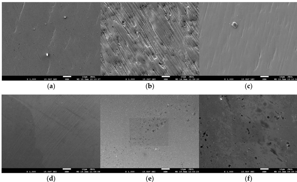
**Figure 7.** SEM images of surface of Ti after potentiodynamic polarization measurements in (a) brackish water, (b) seawater, and (c) seawater bittern; and surfaces of Ti6Al4V after measurements in (d) brackish water, (e) seawater, and (f) seawater bittern.
