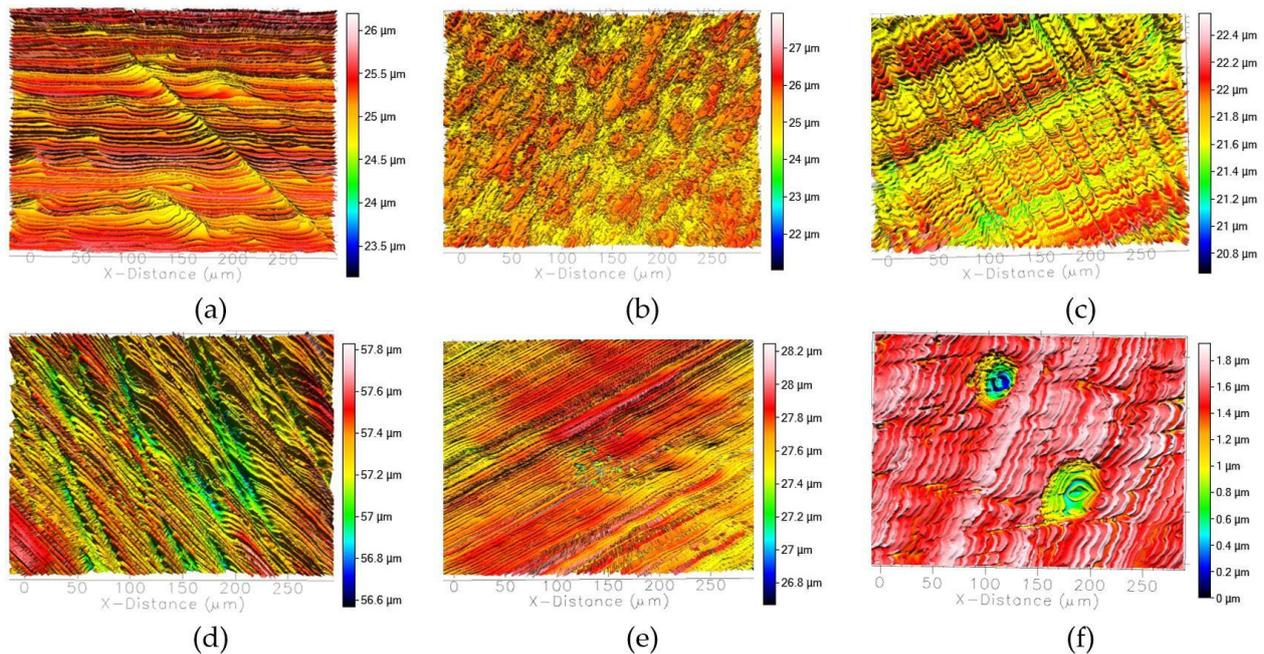
**Figure 10.** Three-dimensional optical profilometry images of surface of = Ti after potentiodynamic polarization measurements in (a) brackish water, (b) seawater, and (c) seawater bittern; and surfaces of Ti6Al4V after measurements in (d) brackish water, (e) seawater, and (f) seawater bittern.
