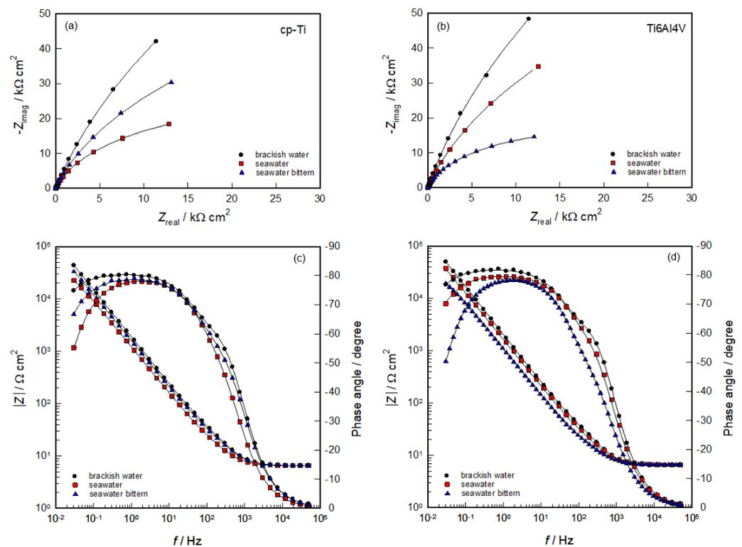
**Figure 4.** Nyquist (a,b) and Bode (c,d) plots recorded on cp-Ti and Ti-6Al-4V alloy in different solutions.
