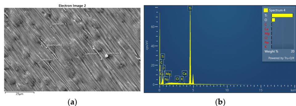
**Figure 8.** (a) SEM image of surface of Ti after potentiodynamic polarization measurements in seawater and (b) EDS point analysis in Spectrum 4.
