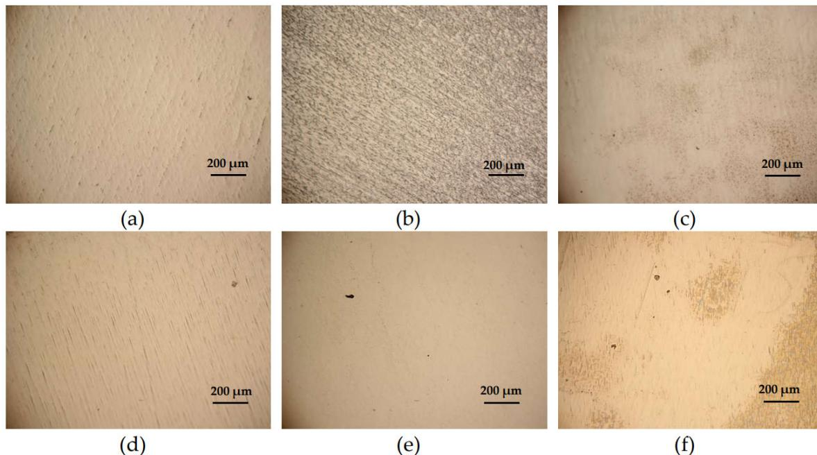
**Figure 6.** Optical microscope images of surface of Ti after potentiodynamic polarization measurements in (a) brackish water, (b) seawater, and (c) seawater bittern; and surfaces of Ti6Al4V after measurements in (d) brackish water, (e) seawater, and (f) seawater bittern.
