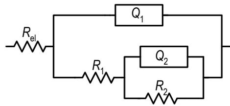
**Figure 5.** The EC model used to fit the EIS data.
