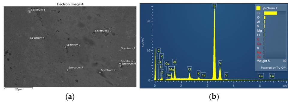
**Figure 9.** (a) SEM image of surface of Ti6Al4V after potentiodynamic polarization measurements in seawater bittern and (b) EDS point analysis in Spectrum 1.
