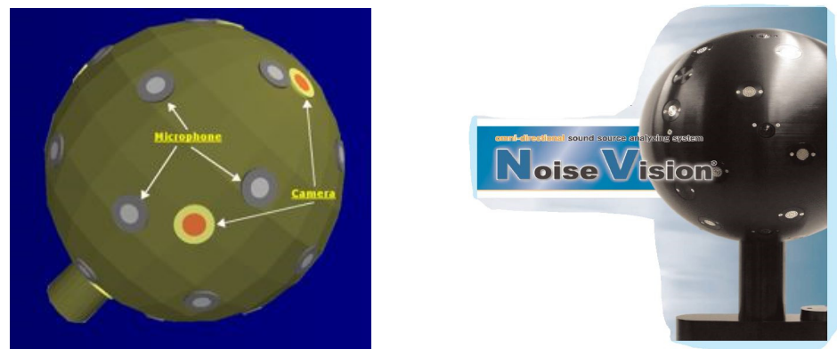
Figure 5. Spherical baffled beamforming sensor with 31 transducers and 12 cameras.
