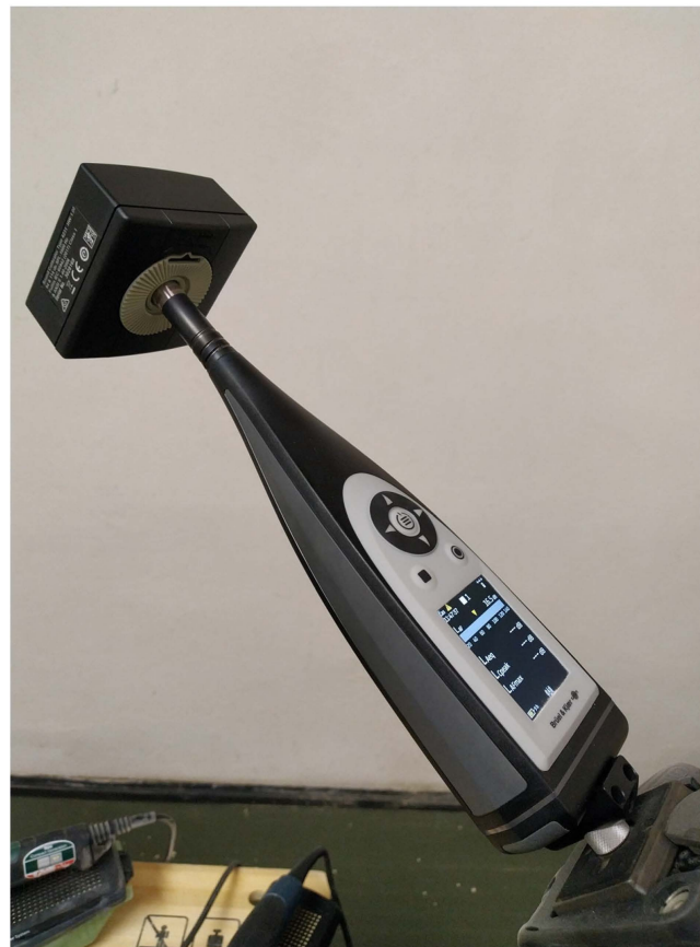
Figure 3. Calibration of integrating-averaging sound level meter.
