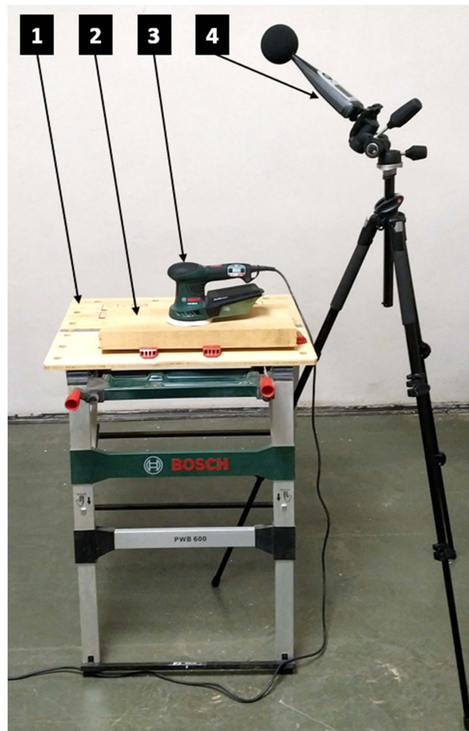
Figure 1. Experimental configuration design: 1—workbench, 2—test specimen, 3—sander, 4—sound level meter.
