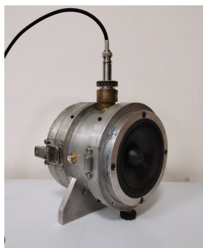
Figure 5. Loudspeaker setup including its back cavity and an internal microphone. The microphone is positioned inside the back cavity to measure the acoustic pressure necessary for determining the speaker's velocity.
