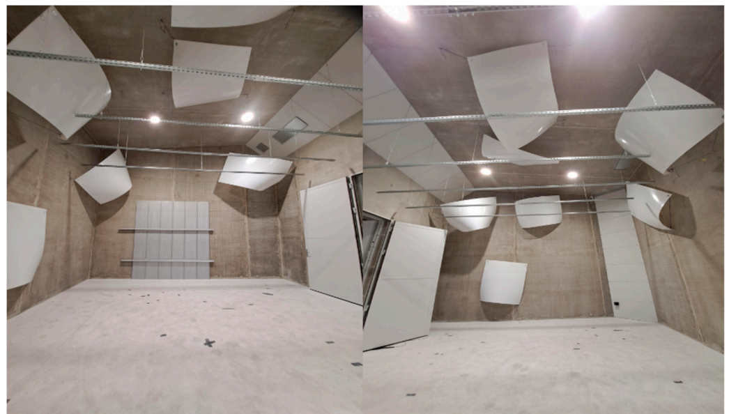
Figure 1. Interior view of the reverberation chamber used during measurements.
