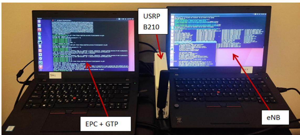
Figure 2. 4G/LTE Base Station Setup.
