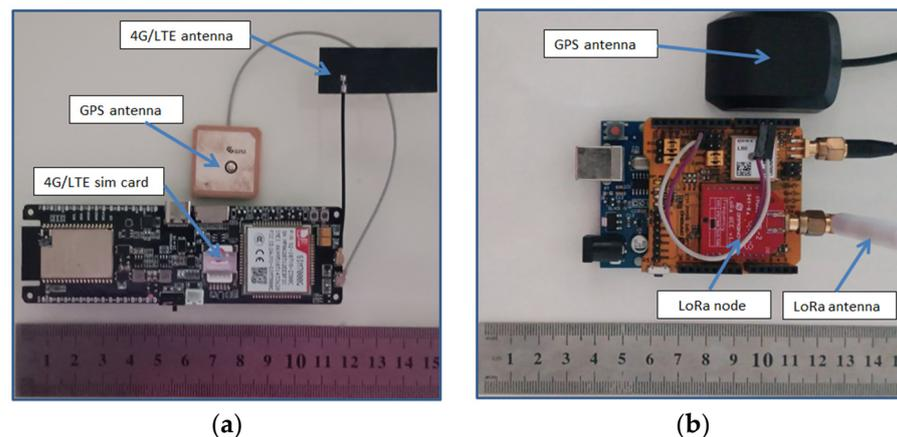
**Figure 3.** (a) 4G/LTE module; (b) LoRa node.
