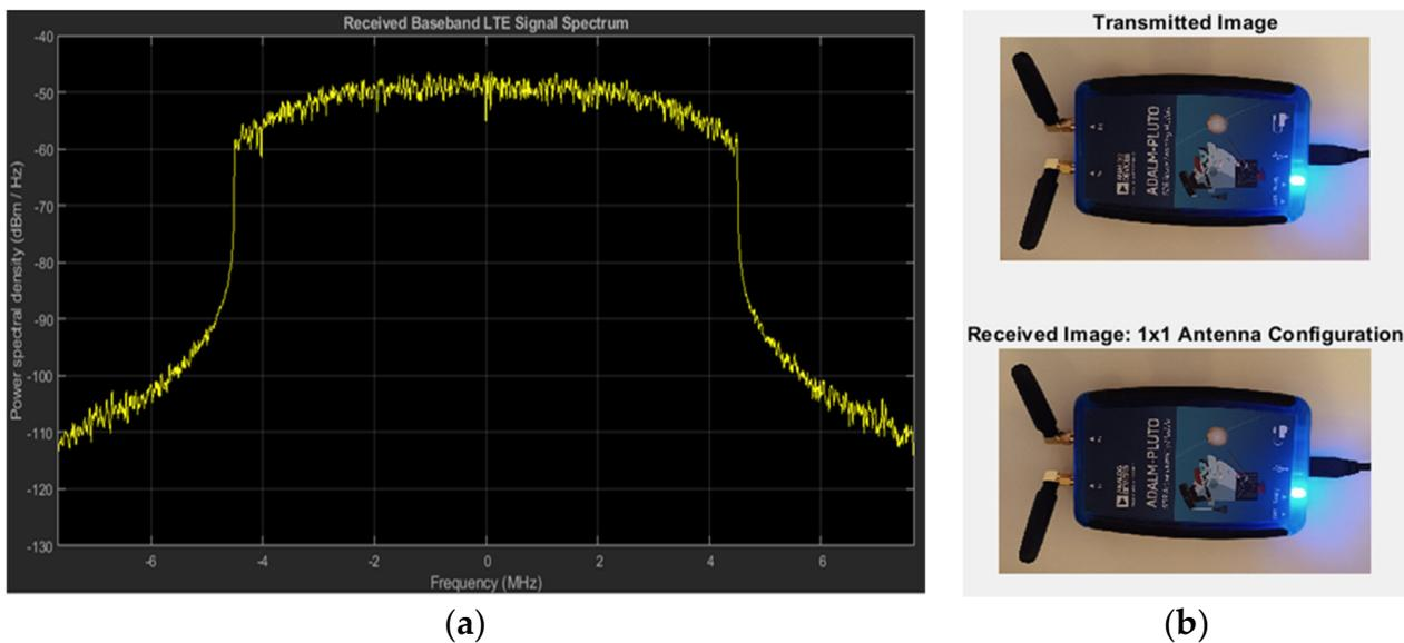
**Figure 9.** (a) Received Baseband LTE Signal Spectrum; (b) Transmitted and Received Image.
