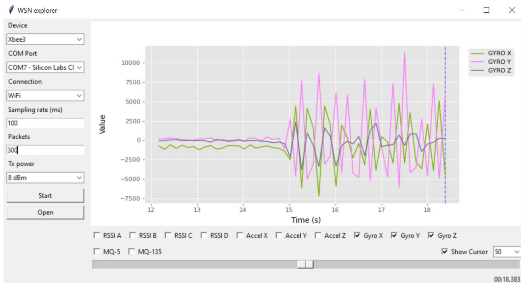
(a) Real-time three-axis acceleration and gyro signals displayed on a graphical user interface.
