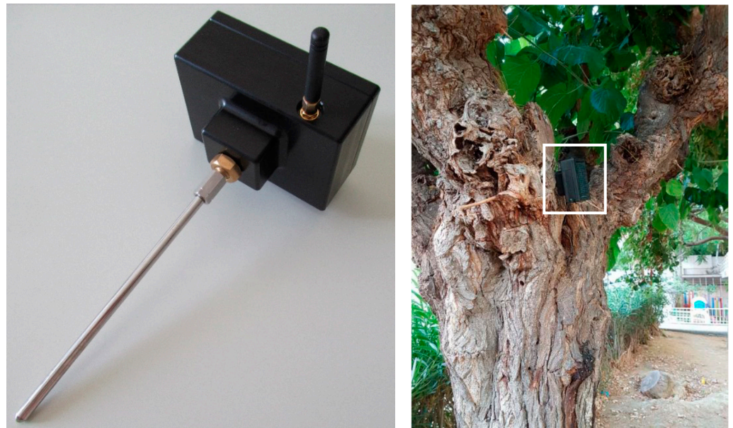
Figure 2. Left: the device is a recorder of vibrations that are picked up by the metal probe. Right: the device attached to a mulberry listening for the cerambycid pest Xylotrechus chinensis .
