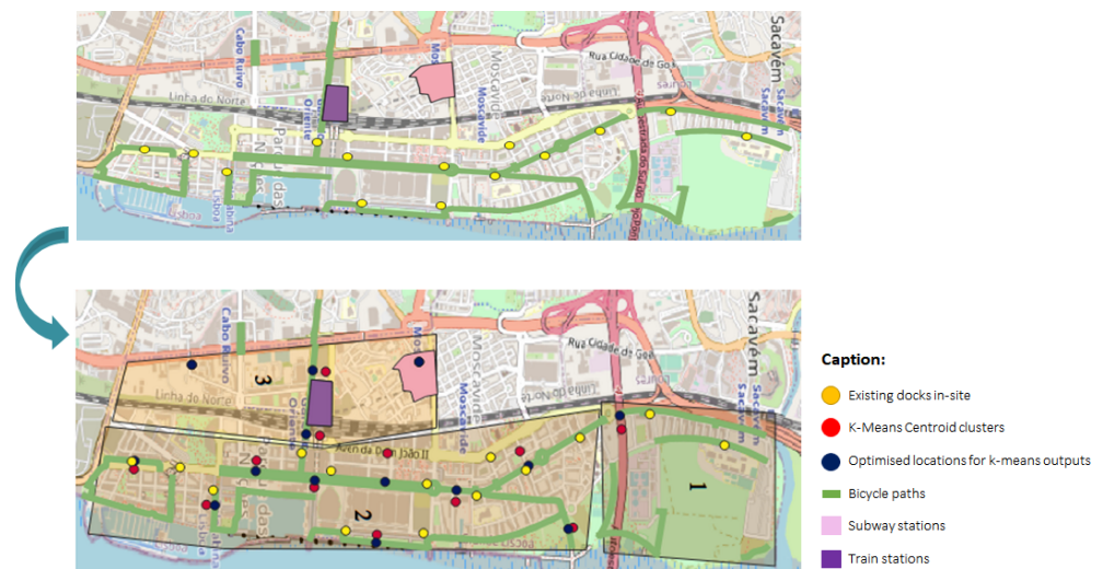
Figure 9. Bike-sharing docking stations in Parque das Nações: Existing docks in-site are represented by yellow dots; red dots represent centroid clusters; dark blue dots represent the optimised locations for K-Means outputs (docking stations over bike paths). Subway has the pink colour polygon, while the purple polygon regards the train station. The map was divided in three segments. Background map source: OpenStreetMap [46].
