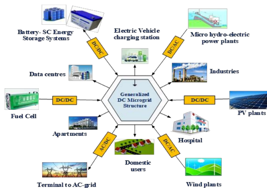
Figure 1. DC microgrid architecture.
