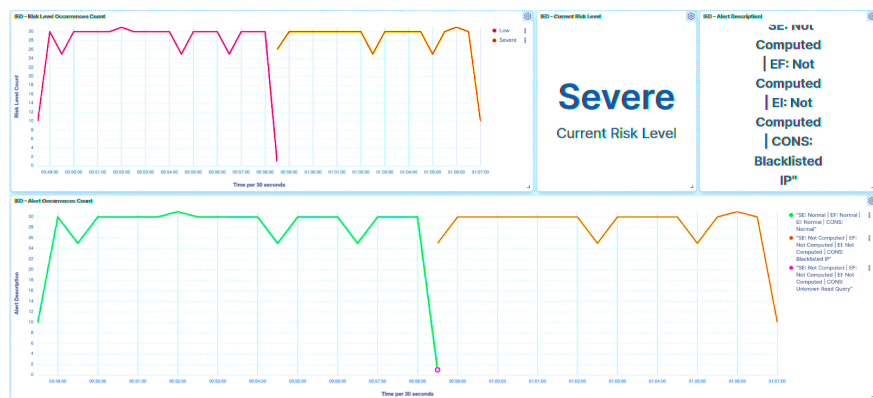
Figure 43. SCADA UI—IED1B: false data injection detection.
