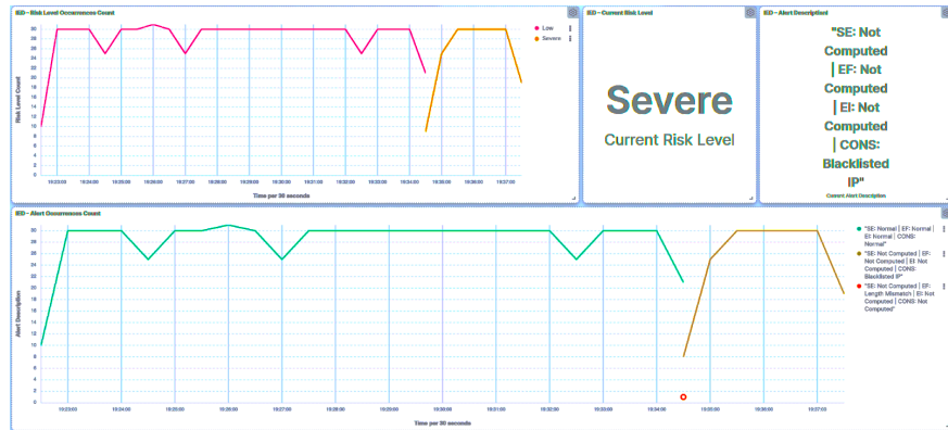
Figure 41. Trust SCADA HMI UI—IED1B: payload injection detection.
