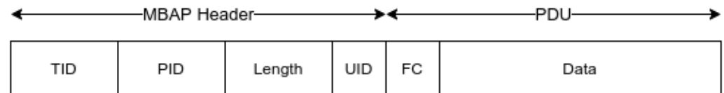
Figure 3. Modbus TCP packet structure.
