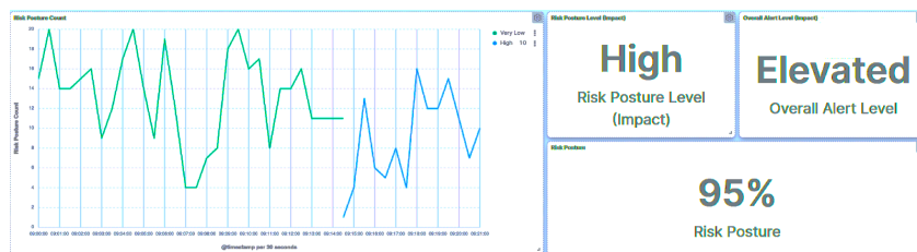
Figure 16. Central agent UI—SCADA: reconnaissance on IED1A.
