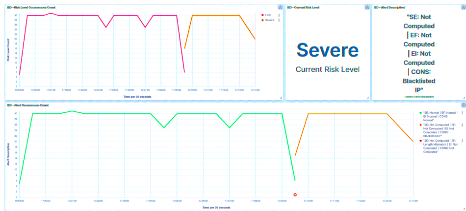
Figure 39. SCADA UI—IED1B: length manipulation detection.
