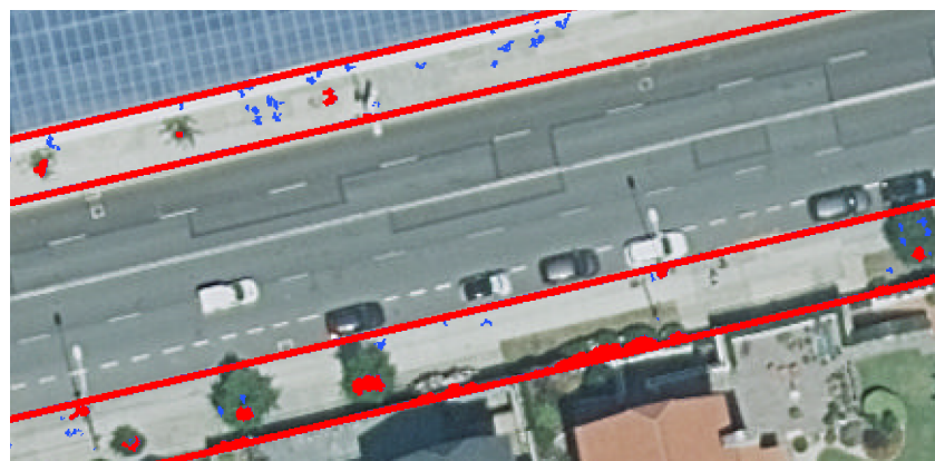
Figure 8. Detail of obstacle surface. Examples of some of the obstacles that have been detected are streetlights and trees. Red pixels show permanent obstacles and blue pixels show pedestrians. Source: self-made.
