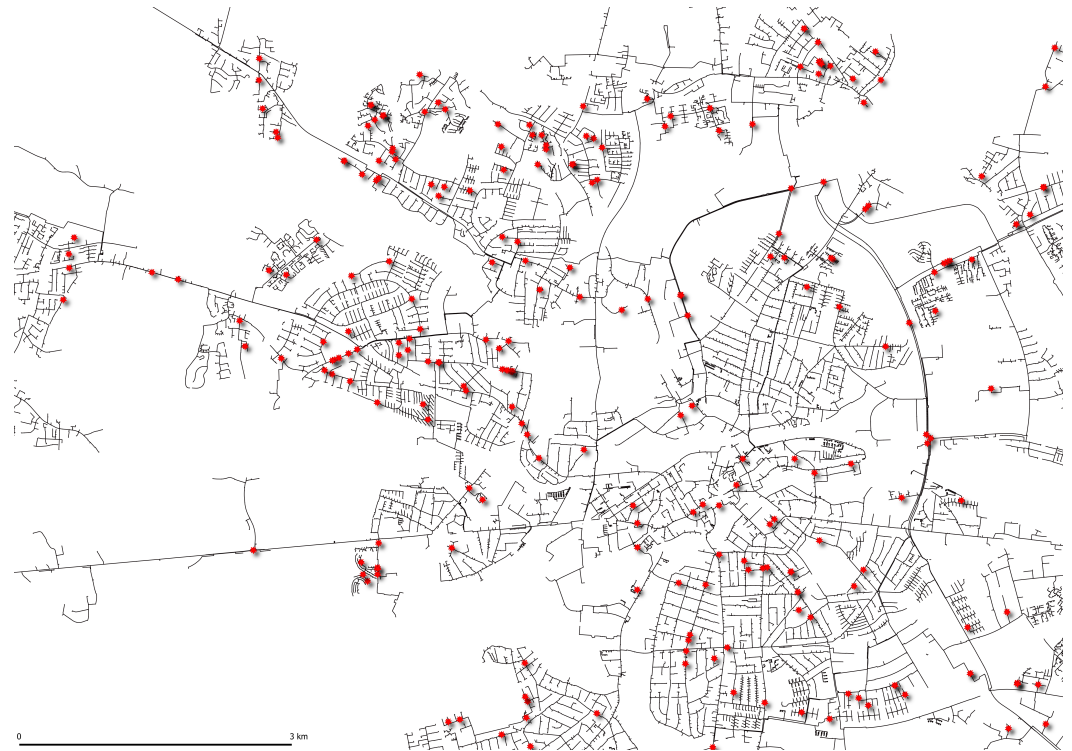
Figure 1. Example of GIS data of the district heating system, including distribution and transmission pipes, and historical thermography reports indicating failures shown as red stars.
