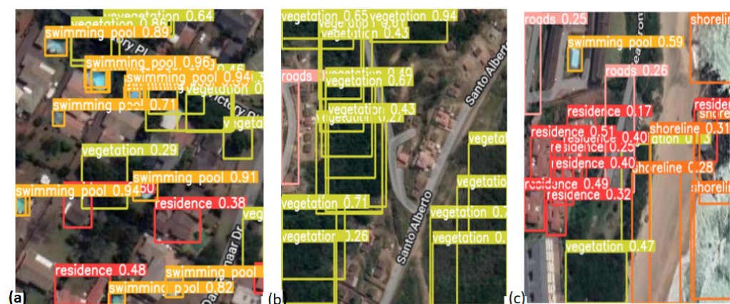
Figure 5. Detecting objects in sample satellite image; (a) Detection of swimming pools and residences; (b) detection of vegetation; (c) detection of residences, roads, and shorelines (Adegun et al. [37]).
