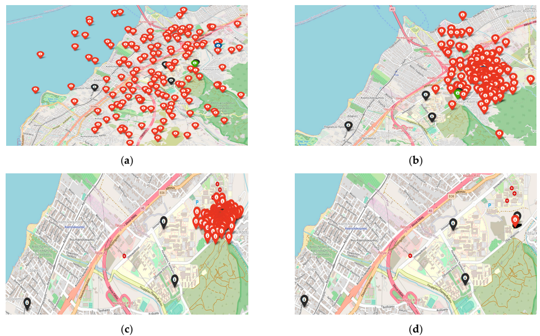
Figure 8. Iterations with our newly introduced, modified SL-PSO. In (a), the initial particles produced are illustrated in red. The best particle is colored blue. In (b), the generated particles after some iterations are in red. In (c), the generated particles after a set of iterations are in red, and finally, in (d), the final specified particle is in red.
