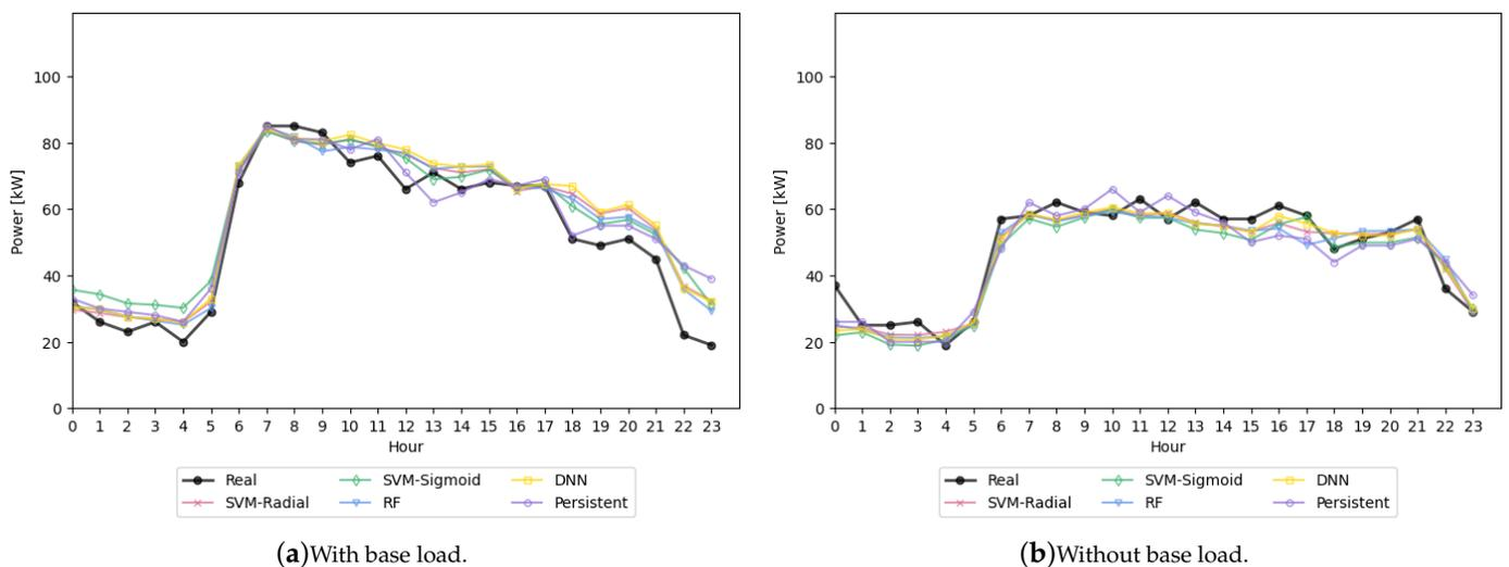
**Figure 9.** Prediction of a day for Industrial building in both (a) with and (b) without base load.
