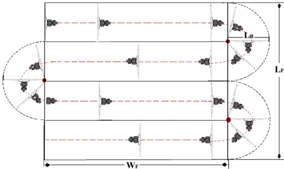
**Figure 2.** Field layout and driving directions of tractor during spraying operation (example with four passes and three half rotations).
