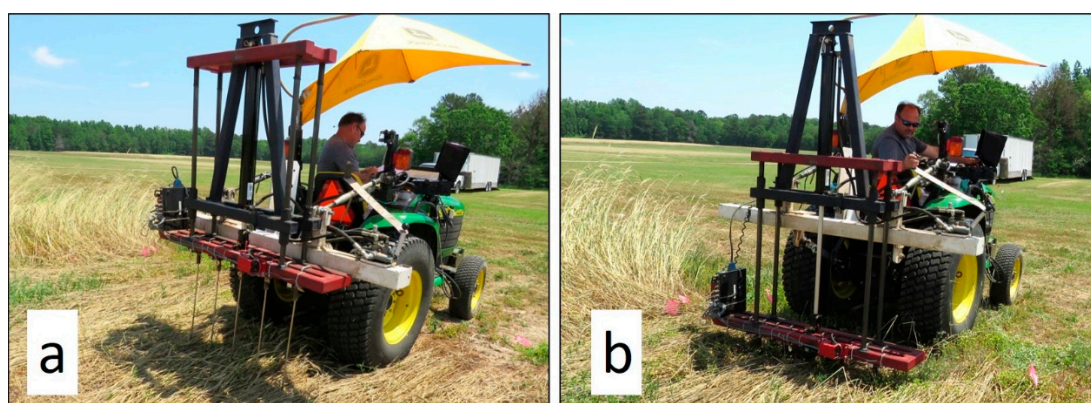
Figure 5. Soil strength measurements by mobile multiple soil cone penetrometer after rolling: (a) before inserting into soil; (b) fully inserted in soil.
