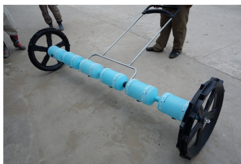
Figure 9. Drum seeder for rice seed sowing. Source: Photo was taken by the author at An Giang province on 5 September 2014.
