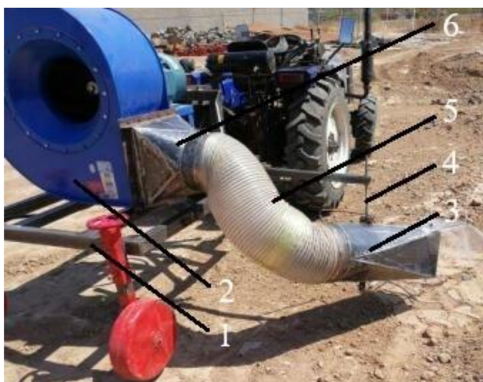
Figure 20. Principle prototype. 1: chassis, 2: centrifugal fan, 3: windpipe, 4: fan outlet transfer tube, 5: hose, 6: windpipe adjustment device.
