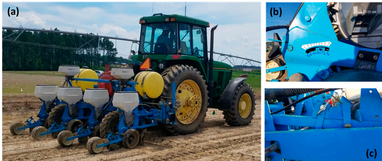
Figure 1. (a) Four-row Monosem NGPlus vacuum precision planter, (b) depth control mechanism, and (c) mechanical downforce assembly used for attaining different downforce adjustments in this study.
