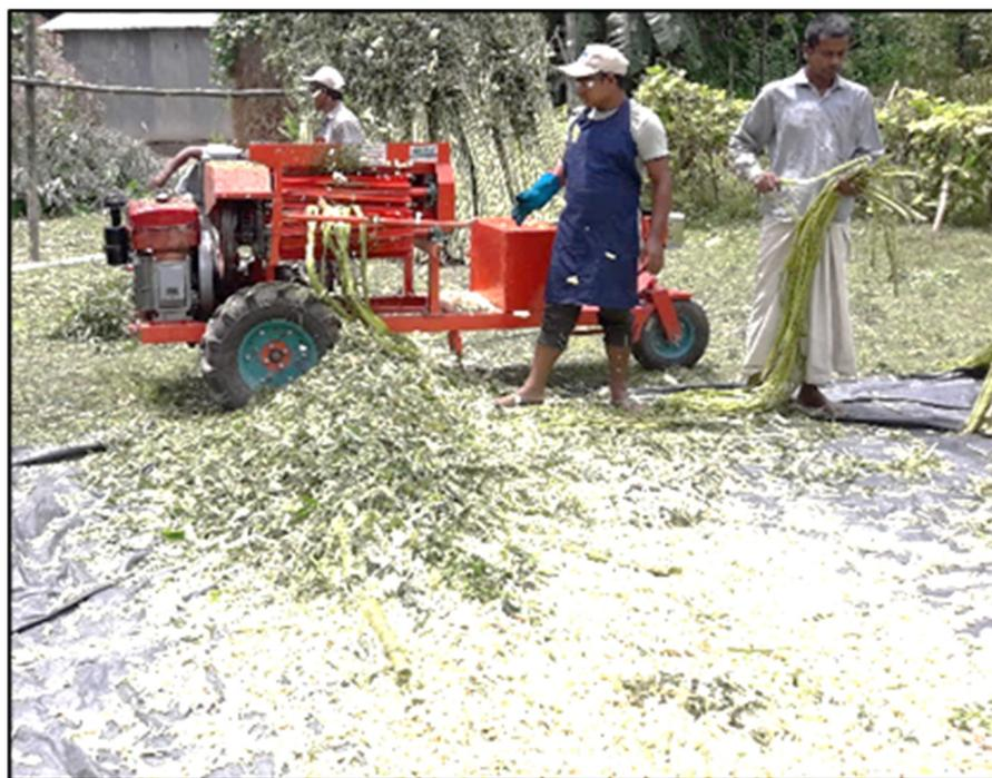
**Figure 11.** Jute fiber extraction by the developed Aashkol.
