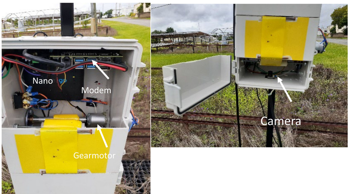
Figure 1. The web-RAID station opened at the top (left) and bottom (right) to see the main components.
