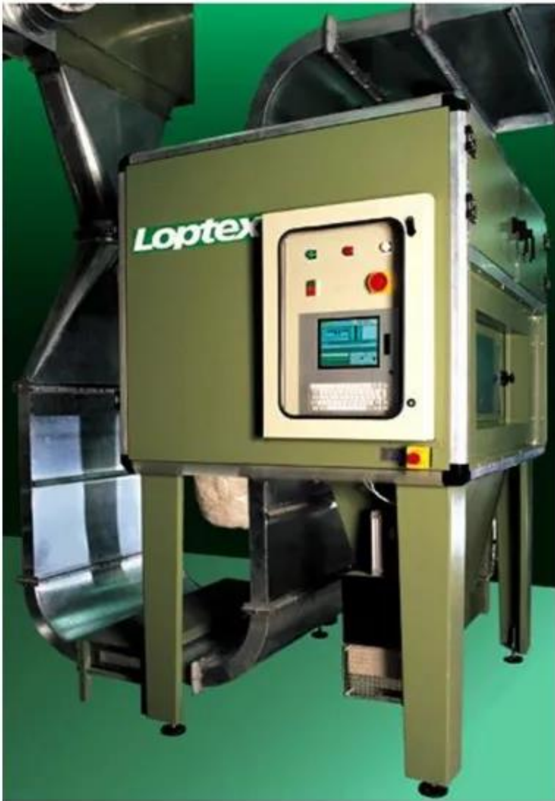
Figure 6. Example Loptex sorter that uses both optical and ultrasonic sensors (adopted with permission from [95]).
