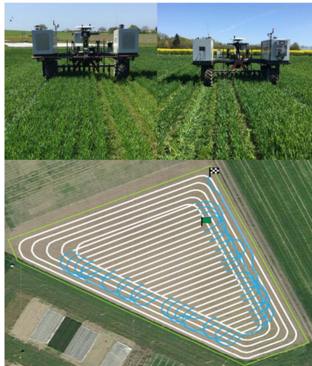
Figure 21. Weeding operation with the robot in a triangle shape field.
