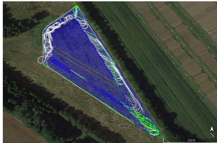
Figure 2. An example of analysis for the robot's in-field operation. "Manual driving": When the robot drives manually by the robot's operator (Green color). "Automatic and working": When the robot automatically performs the operation in the field (Blue color). "Automatic and not working": When the robot automatically moves but not performing the operation for example when it turns in the headland part (White color).
