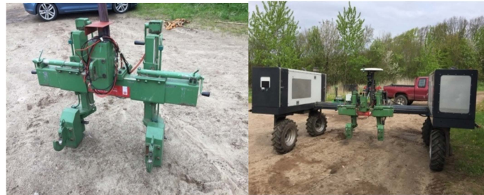
Figure 3. Mounted string gauge on the robot.
