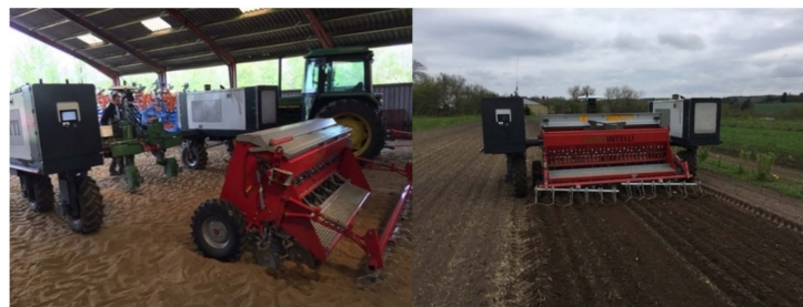
Figure 4. Grain drill seeder, 3 (m)/25 rows, 5 (km/h), 4 (cm) depth. The seeder was filled with weights in the center to represent the weight of the seed. Total weight 210 (kg) ( 4 \times 30 (kg) + 2 \times 45 (kg)).
