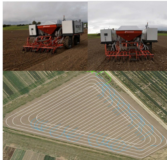
Figure 9. Seeding operation with the robot in a small triangle field.
