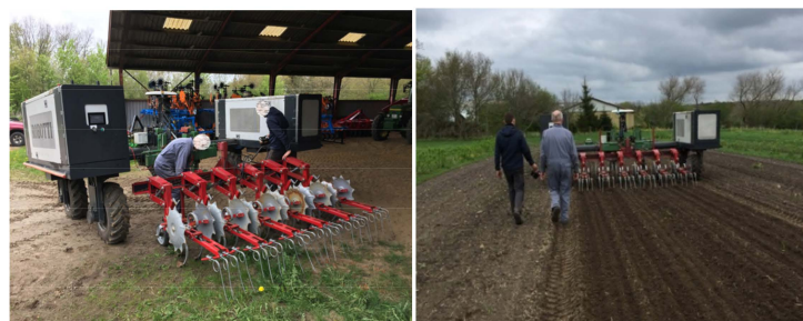
Figure 5. Mechanical weeder (Rod weeder), 3 (m), 5 (km/h), 2 (cm) depth.
