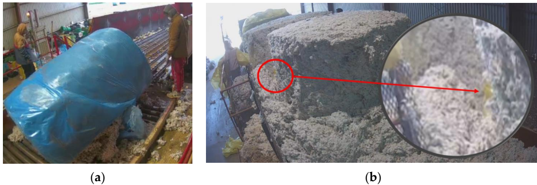
Figure 1. Module feeder floor system: (a) unloading of round module onto module feeder floor; (b) where module accidentally tipped over trapping plastic underneath it so that the crew couldn't remove the tail. Whenever this situation occurred, the gin crew wasn't always able to remove all the plastic before it went into the gin.
