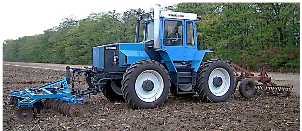
Figure 1. Machine–tractor unit for strip-till two-pass technology implementation.
