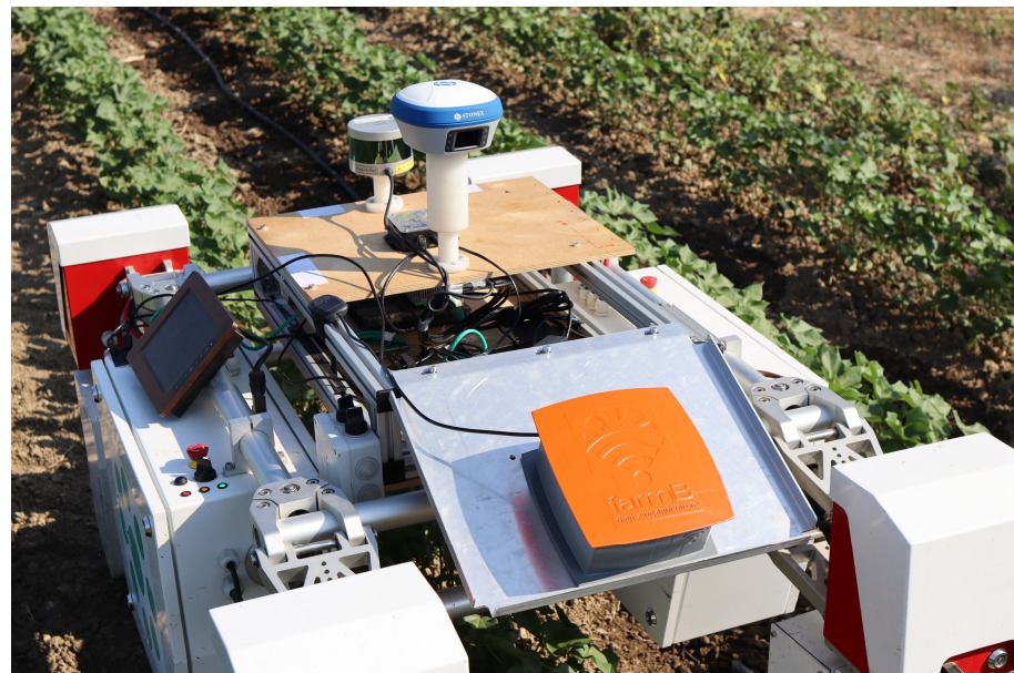
Figure 7. The second implemented UGV (Thorvald) for the system demonstration.
