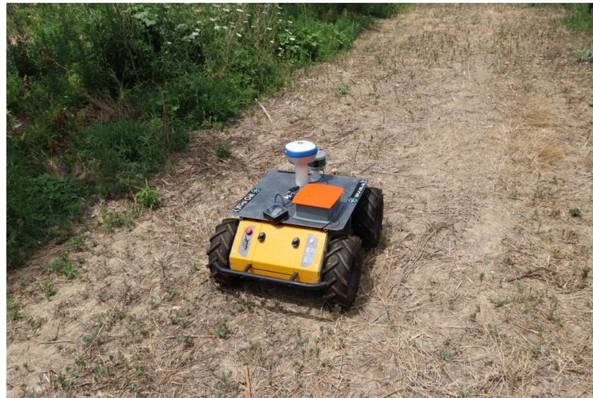
Figure 6. The first implemented UGV (Husky) for the system demonstration.
