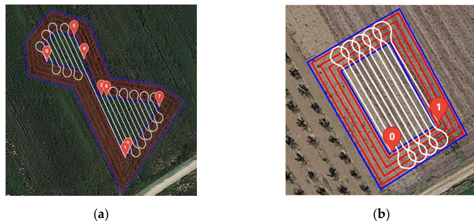
Figure 3. Headland passes (red) and inner boundary (blue) after (a) automatic reduction and (b) automatic increase.
