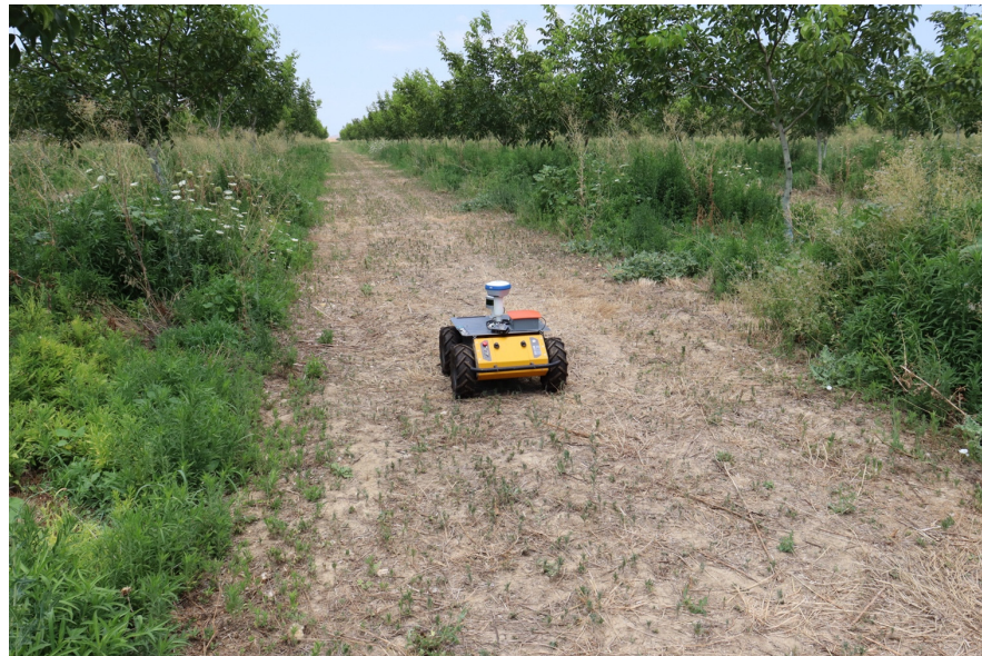
Figure 13. Husky following a track in the middle of the row.
