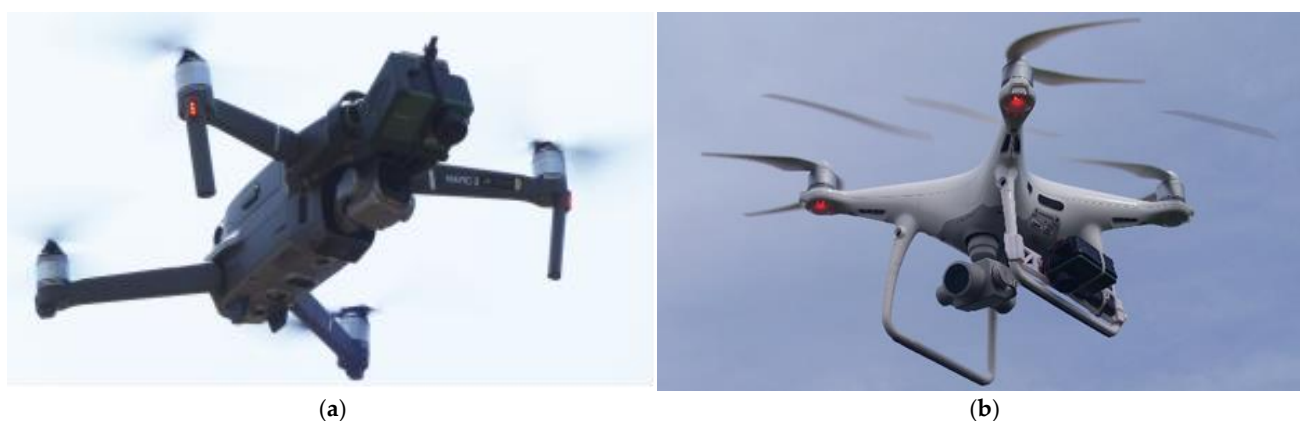
Figure 1. UAV DJI Mavic 2 Pro, MAPIR Survey3W Camera (a). DJI Phantom 4 Pro, MAPIR Survey3W Camera (b).
