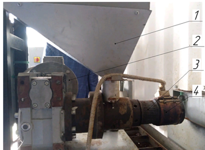
Figure 4. General view of the laboratory screw press: 1—receiving bin; 2—electric drive; 3—extracting box; 4—heating element to maintain the temperature of the press.
