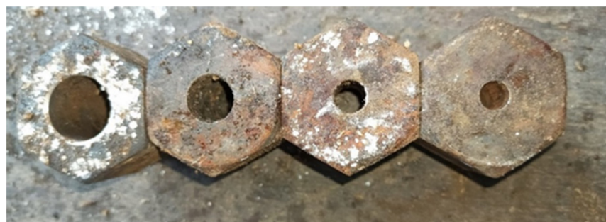
Figure 1. Replaceable nozzles with variable diameter for cake outlet.
