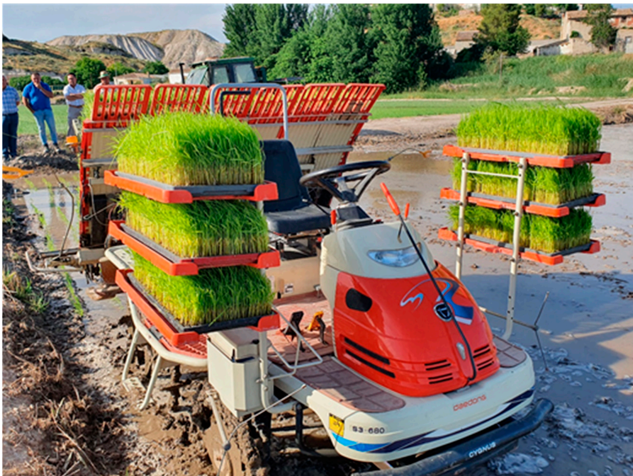
Figure 1. Rice transplanting machine. On the sides of the machine are nursery trays with young rice plants ready for transplantation. At the back, an automatic transplanting mechanism picks up the seedlings with mechanical forks and carefully places them into the soil.
