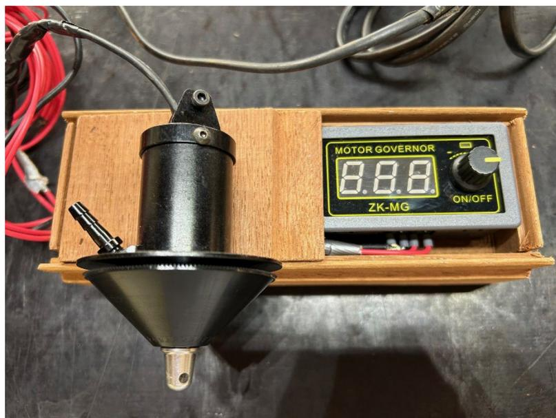
**Figure 2.** Control of nozzle rotation through a pulse width modulation (PWM) pulse generator. Source: authors (2024).
