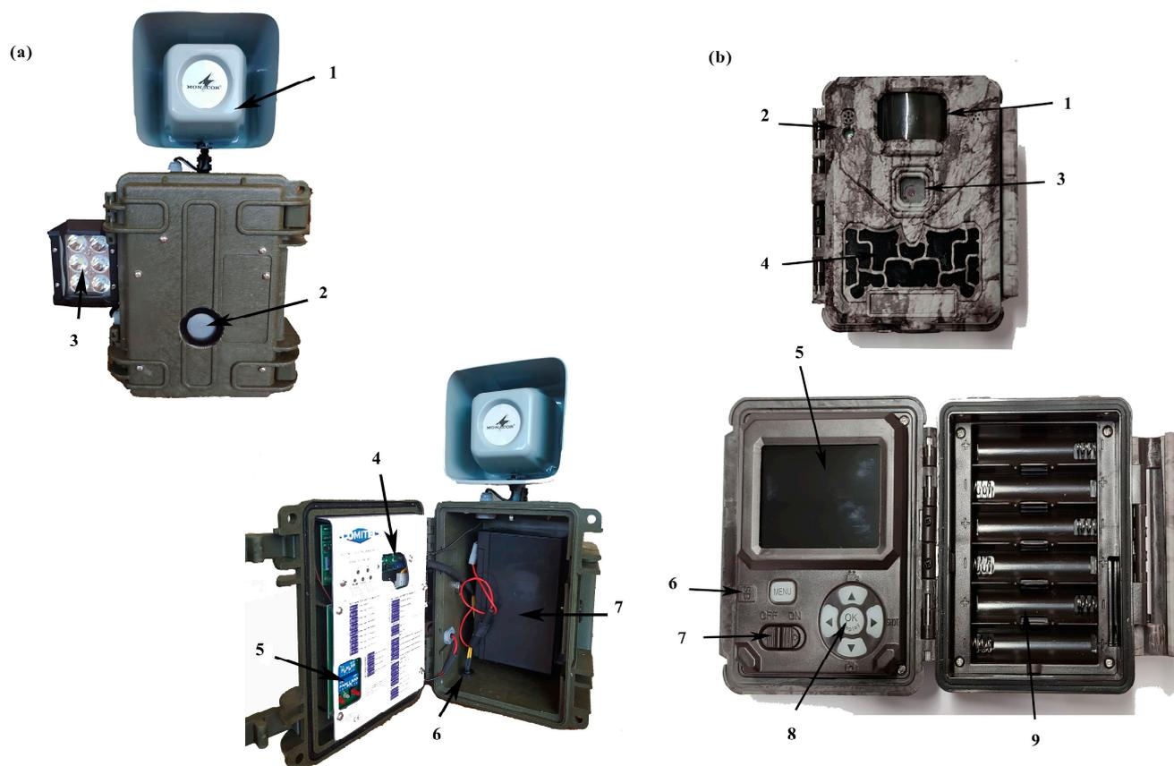
**Figure 2.** Playback device (a) components: Speaker (1), PIR sensor (2), six high-power LED illuminators (3), power switch and volume–tone adjustment button (4), DIP switch programming and electronic circuit in mp3 with SD card slot (5), integrated socket for solar panel (6), 12-volt battery (7). Camera trap (b) components: PIR sensor (1), LED indicator (2), lens (3), IR LED (4), display screen (5), SD card slot (6), on/off switch (7), operation buttons (8), battery case (9).
