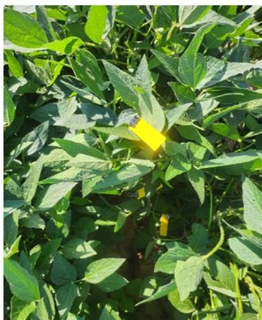
**Figure 3.** Soybean plant showing top, middle, and bottom placement of water-sensitive cards.
