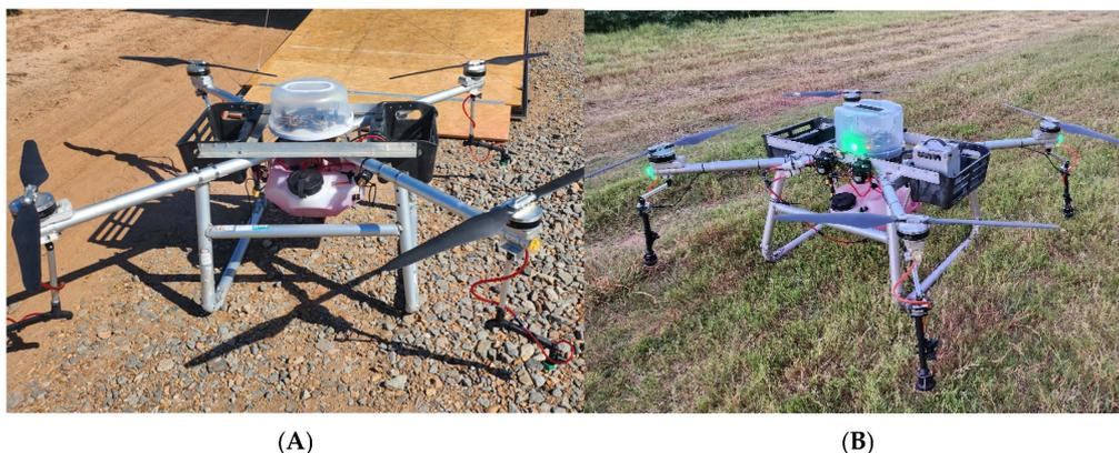
**Figure 1.** Spray drones used in the test mounted with (A) standard hydraulic orifice system and (B) centrifugal/rotary spray system.
