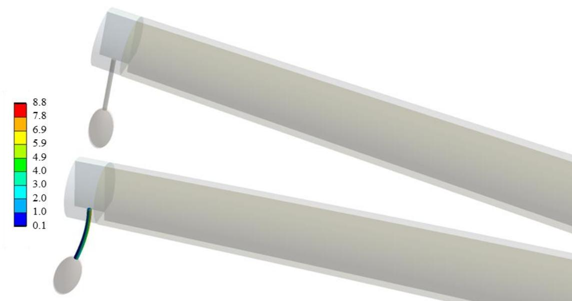
**Figure 15.** Stress predicted by the harmonic analysis in the olive stem, evaluated at the shaking frequency. Values in MPa.
