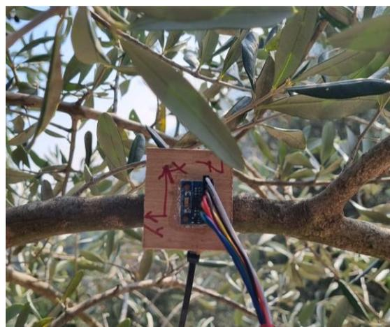
**Figure 7.** Triaxial accelerometer applied near the branch tip. Local accelerometer  $y$ -axis was aligned with the local branch axis.
