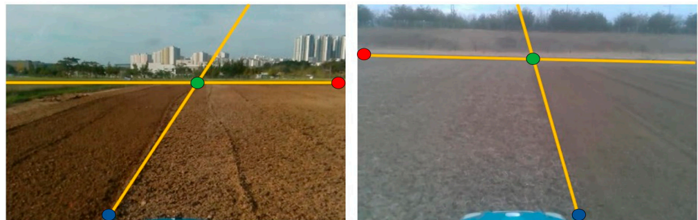
Figure 1. Visualization of three landmark points for the tillage boundaries: The line connecting the red and green points indicates the direction of travel, while the green and blue points mark the positions for the tractor's U-turn.
