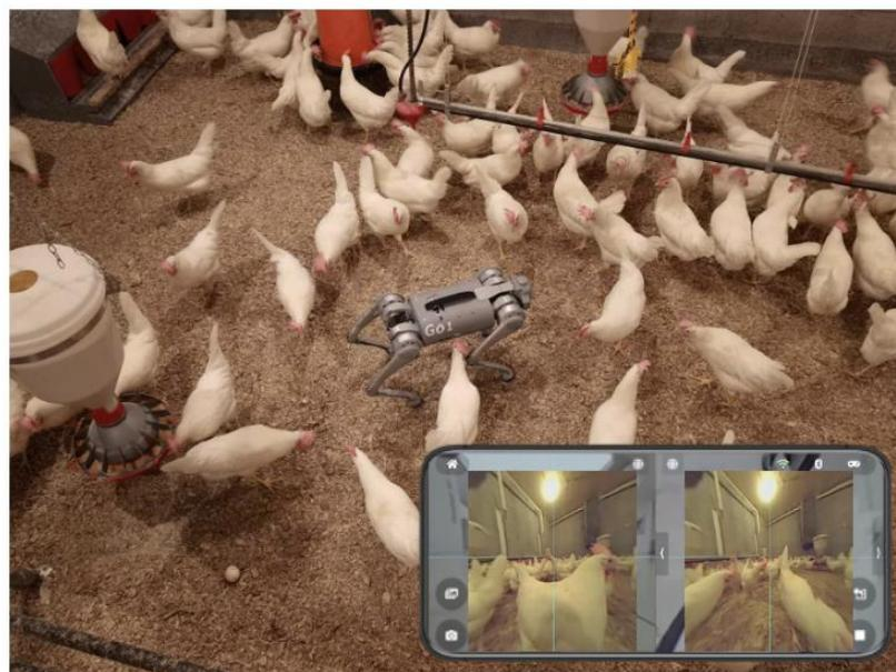
Figure 3. The robot dog in walking mode collecting chicken and egg images in the research poultry house.
