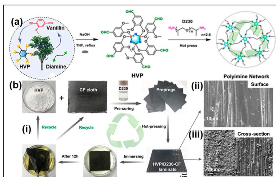
**Figure 10.** (a) Synthesis procedure of polyimine vitrimer; (b) formation of HVP/D230-CF composite and its upcycling (i), and SEM image (ii) surface and (iii) cross-section [reproduced with permission from Liu et al.; published by Elsevier, 2021] [51].
