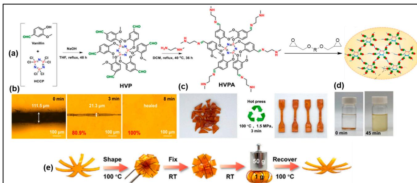
**Figure 16.** (a) Synthesized way of imine bond containing hardener (HVPA) from vanillin and its cured network; repairability (b), reprocessability (c), degradability (d), and reformability (e) of the cured thermoset [reproduced with permission from Peng et al.; published by Elsevier, 2022] [79].
