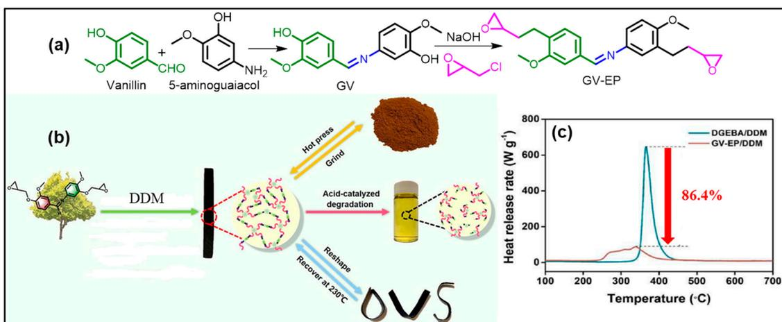
**Figure 6.** (a) Synthesized of greener Schiff-base epoxy monomer (GV-EP); (b) curing process and its physical reprocessing, chemical degrading and reshaping performance; (c) pHRR versus temperature curve for the developed and control thermosets from the cone calorimeter test [reproduced with permission from Li et al.; published by Elsevier, 2022] [52]. Red arrow used for the difference of heat release rate between two thermosets.
