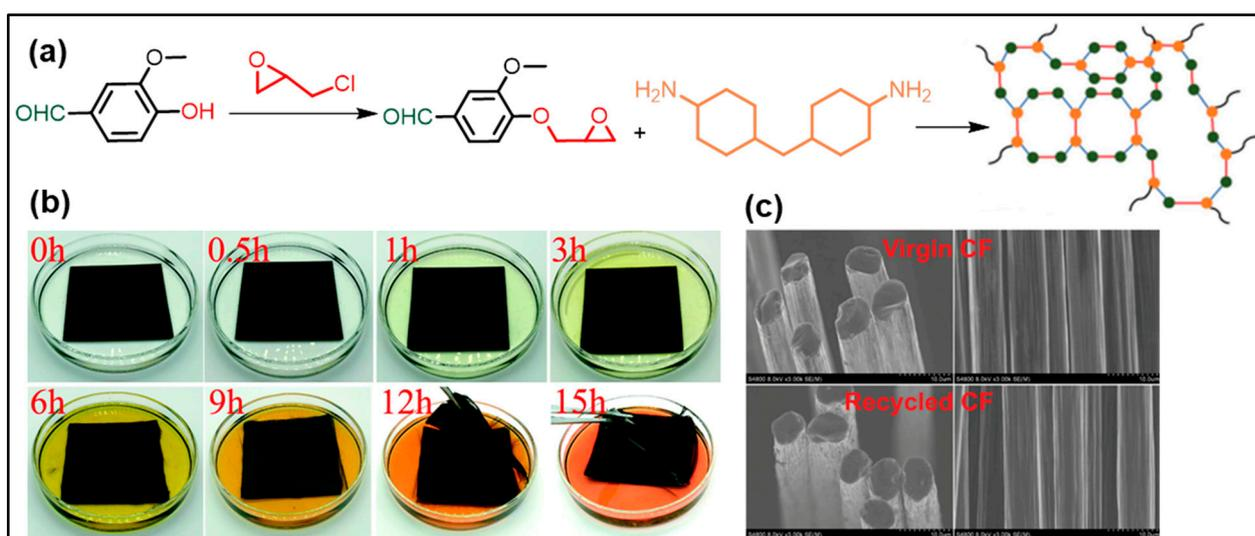
**Figure 5.** (a) Preparation way of epoxy vitrimer, (b) epoxy thermoset decomposition in 0.1 M HCl solution (methanol/H<sub>2</sub>O = 8/2, V/V) at normal temperature for the recovery of carbon fibers from CFRCs, and its SEM images (c) [reproduced with permission from Wang et al.; published by RSC, 2019] [59].
