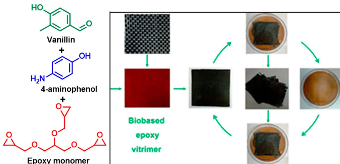
**Figure 15.** Synthesis way of vanillin-modified vitrimer and full recycling of carbon fiber reinforced composite (CFRP) [reproduced with permission from Liu et al.; published by ACS, 2021] [78].
