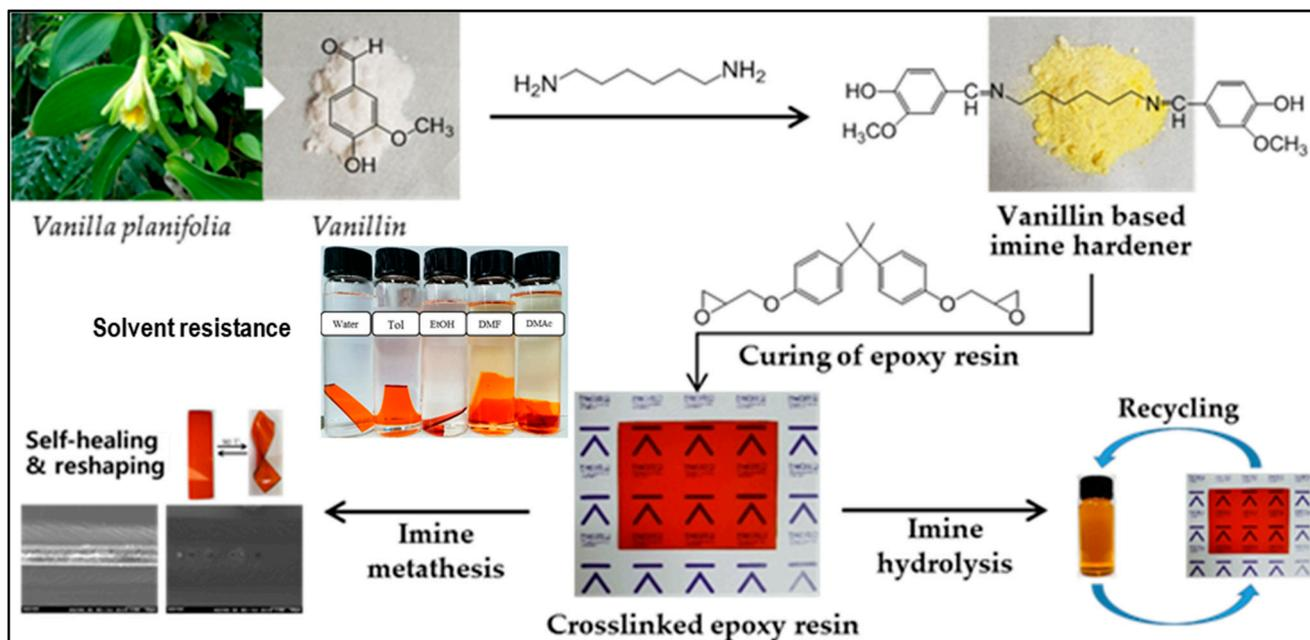
**Figure 12.** Synthesis pathway and properties of healable, reusable, and solvent-stable epoxy vitrimers from imine bonds-containing vanillin-modified curing agent and DGEBA [reproduced with permission from Mai et al.; published by MDPI, 2019] [54].
