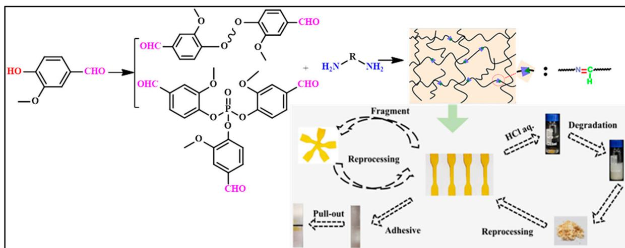
**Figure 18.** Synthesized routes of completely biobased reversible polyimine vitrimer from sustainable vanillin and amine, and its thermal and chemical recyclability [reproduced with permission from Zhou et al.; published by ACS, 2020] [13].
