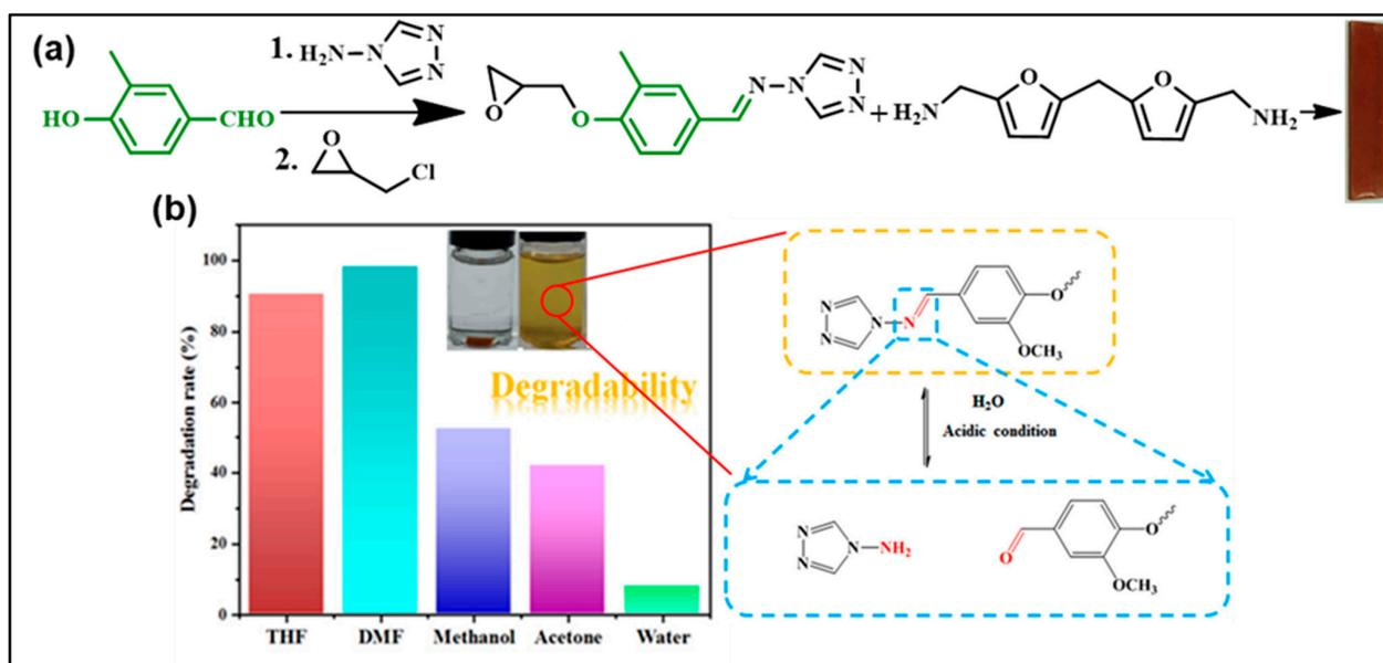
**Figure 19.** (a) Vanillin-modified epoxy monomer (VTA-EP) and its thermoset synthesis pathway, (b) degradability of fully green vitrimer (VTA-EP/DFA) at different solvents and its degradation mechanism [reproduced with permission from Nabipour et al.; published by Elsevier, 2021] [82].
