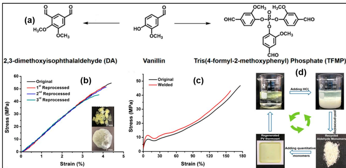
**Figure 20.** (a) Synthesized pathway of aldehyde from vanillin; mechanical recycling (b) and weldability (c) performance; and (d) closed-cycle chemical recycling [reproduced with permission from Hong et al.; published by ACS, 2022] [83].
