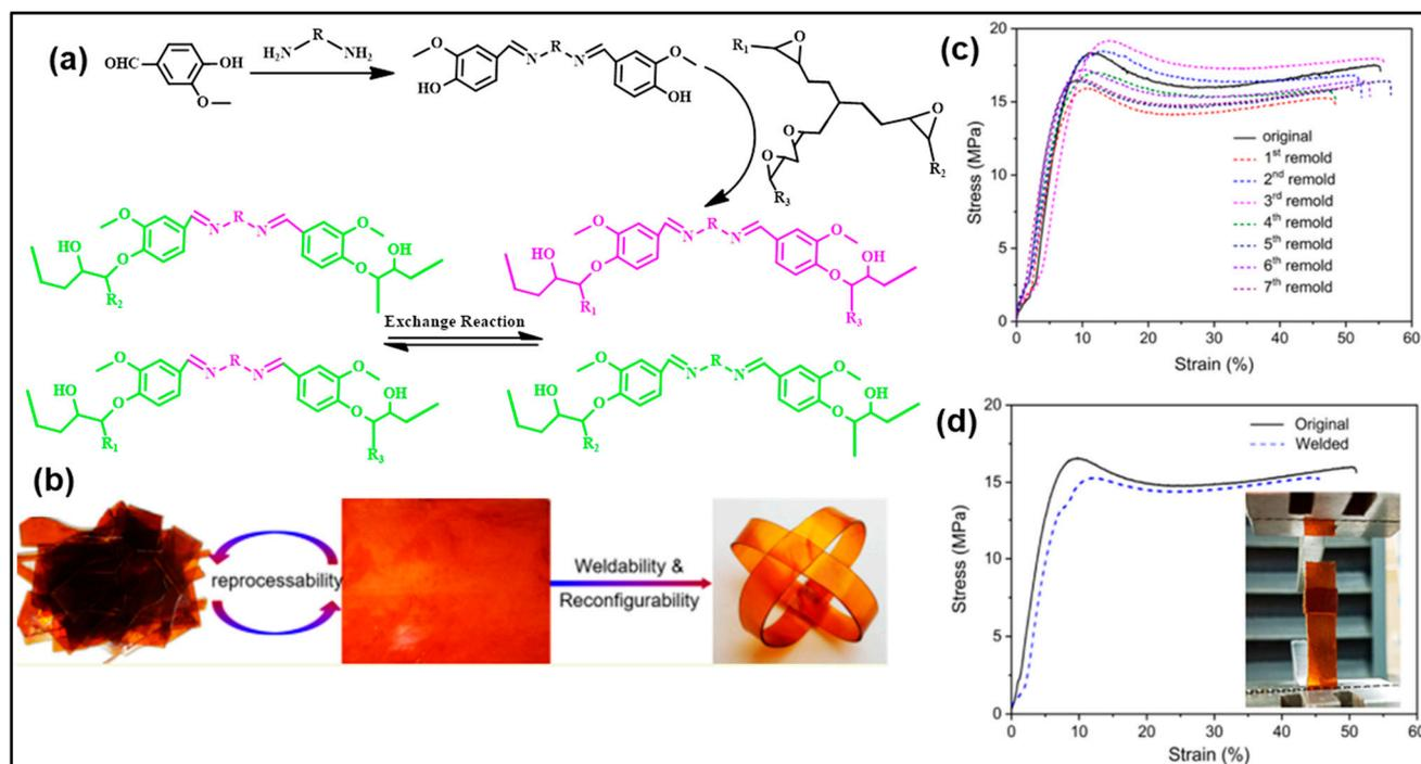
**Figure 17.** (a) Preparation of fully bio-based vitrimers from ESO and vanillin modified (VSB) hardener and its exchange reaction; (b) reprocessability and weldability, (c,d) mechanical strength of pristine and remolded or welded samples [reproduced with permission from Zhao et al.; published by ACS, 2020] [81].
