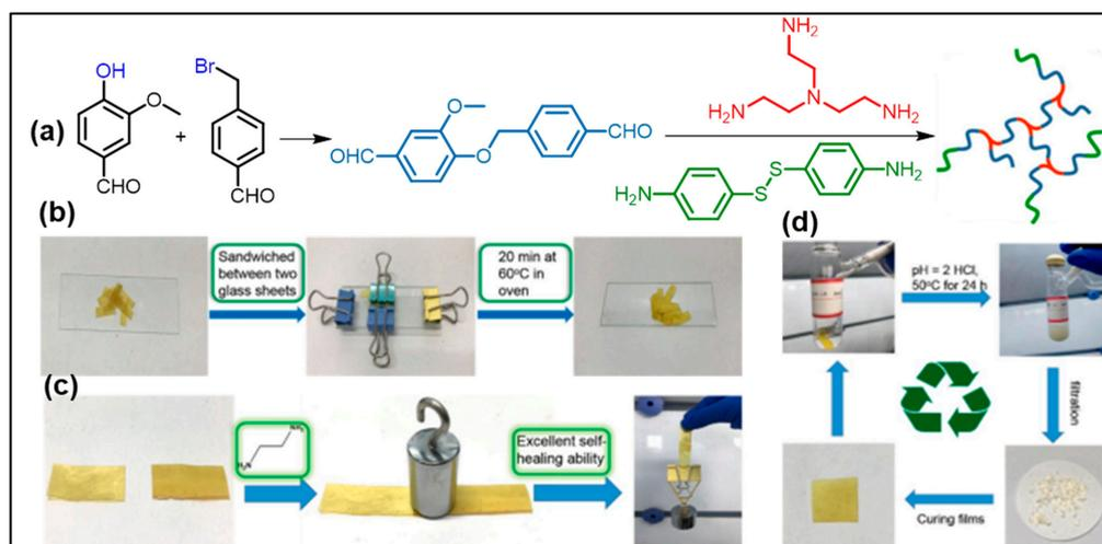
**Figure 8.** (a) Synthesis pathway of vanillin vitrimer; (b) mechanical regeneration of finely ground vitrimers; (c) self-healing performance of the cut samples that could sustain 500 g of load; and (d) chemical reprocessing of the cured vitrimers [reproduced with permission from Guo et al.; published by Elsevier, 2020] [69].
