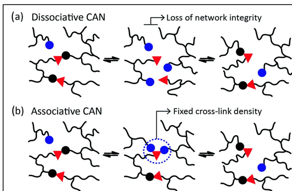
**Figure 2.** Recyclable mechanism of dynamic covalent adaptable networks (DCANs) [Reproduced with permission from Du Prez et al.; published by RSC, 2016] [21]. Blue and black dots, red triangles are used as active functional groups that can react each other at different conditions.
