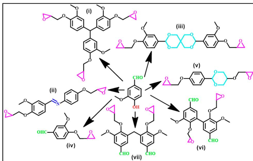
**Figure 3.** Potential modification of vanillin monomer to epoxy monomer.
