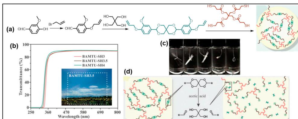
**Figure 9.** (a) Synthesis way of acetal bond-containing vanillin vitrimer; transparency (b), degradability (c) and its mechanism (d) of acetal bond-containing cured vitrimer [reproduced with permission from Ge et al.; published by RSC, 2021] [74].
