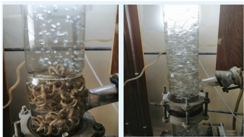
Figure 4. The contact between the ozone gas and the wastewater mixture in a bubble column reactor using two types of packing materials.
