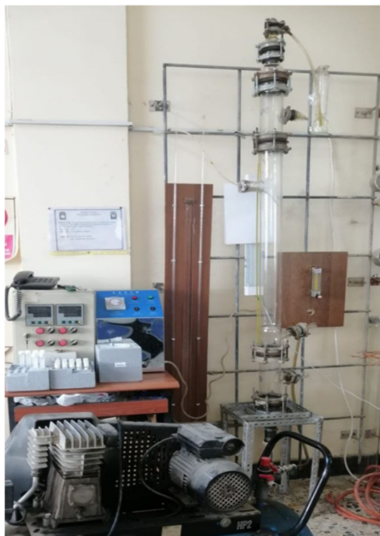
Figure 2. Photograph of the ozonized bubble column reactor apparatus.
