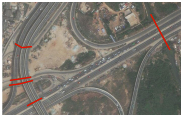
Figure 9. Red lines show four digitized hydro-conditioning features (left) where infrastructures are elevated above ground levels and one (right) where a stream underpasses the infrastructure.
