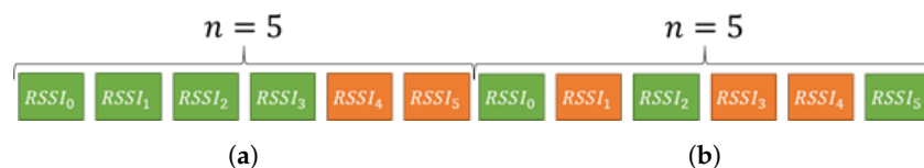
Figure 10. (a) Case where the adversary starts transmitting right after the legitimate node terminated its transmission; (b) The adversary gains access to the channel while the legitimate node has not finished transmitting all of its frames.
