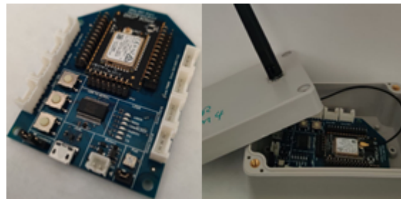
Figure 7. Digi XBee 3 Series programmable module implementing IEEE 802.15.4. in a weatherproof secure enclosure protecting the devices from the elements when deployed.
