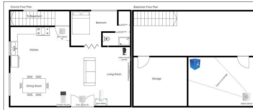
Figure 2. Location of security sensors for the burglary scenario.
