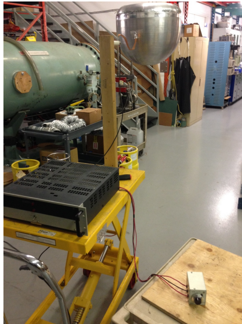
Figure 4. Acorn in the low-voltage configuration. The flexible copper braid connecting the power supply to the acorn is visible.
