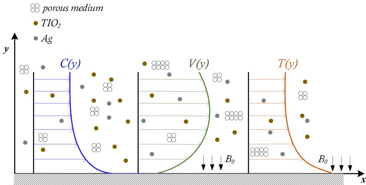
**Figure 1.** The mathematical model of HNF with boundary condition. Concentration,  $C$ , velocity,  $V$ , and temperature,  $T$ , profiles in ( $x$ - $y$ ) space.  $B_0$  is the magnetic field with the direction shown by arrows.
