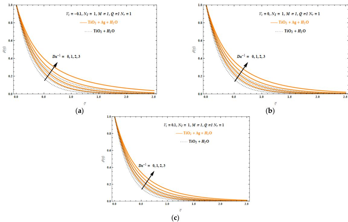
**Figure 11.** Temperature profiles,  $\theta(\eta)$ , versus similarity variable,  $\eta$ , for various  $Da^{-1}$  values,  $N_I = N_r = M = Q = 1$ , and (a)  $V_c = 0.1$ , (b)  $V_c = 0$ , and (c)  $V_c = -0.1$ .
