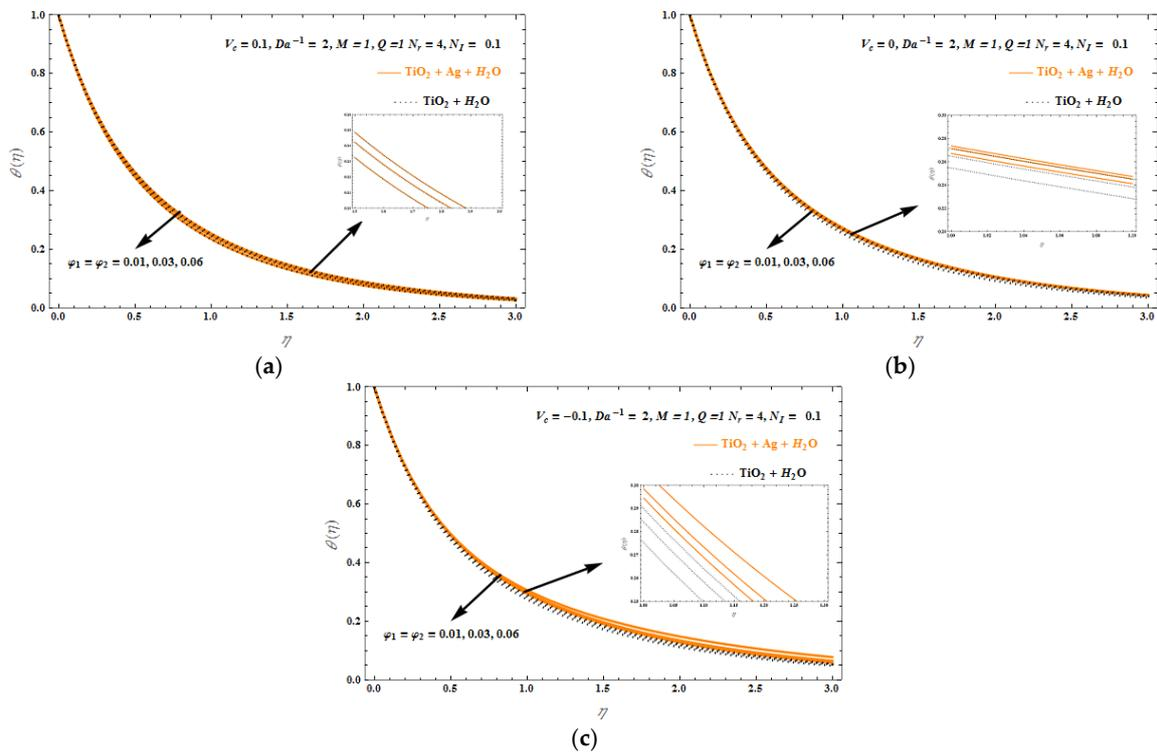
**Figure 12.** Temperature profiles,  $\theta(\eta)$ , versus similarity variable,  $\eta$ , for various  $\varphi_1, \varphi_2$  values,  $Da^{-1} = 2, N_l = 0.1, N_r = 4, M = Q = 1$ , and (a)  $V_c = 0.1$ , (b)  $V_c = 0$ , and (c)  $V_c = -0.1$ .
