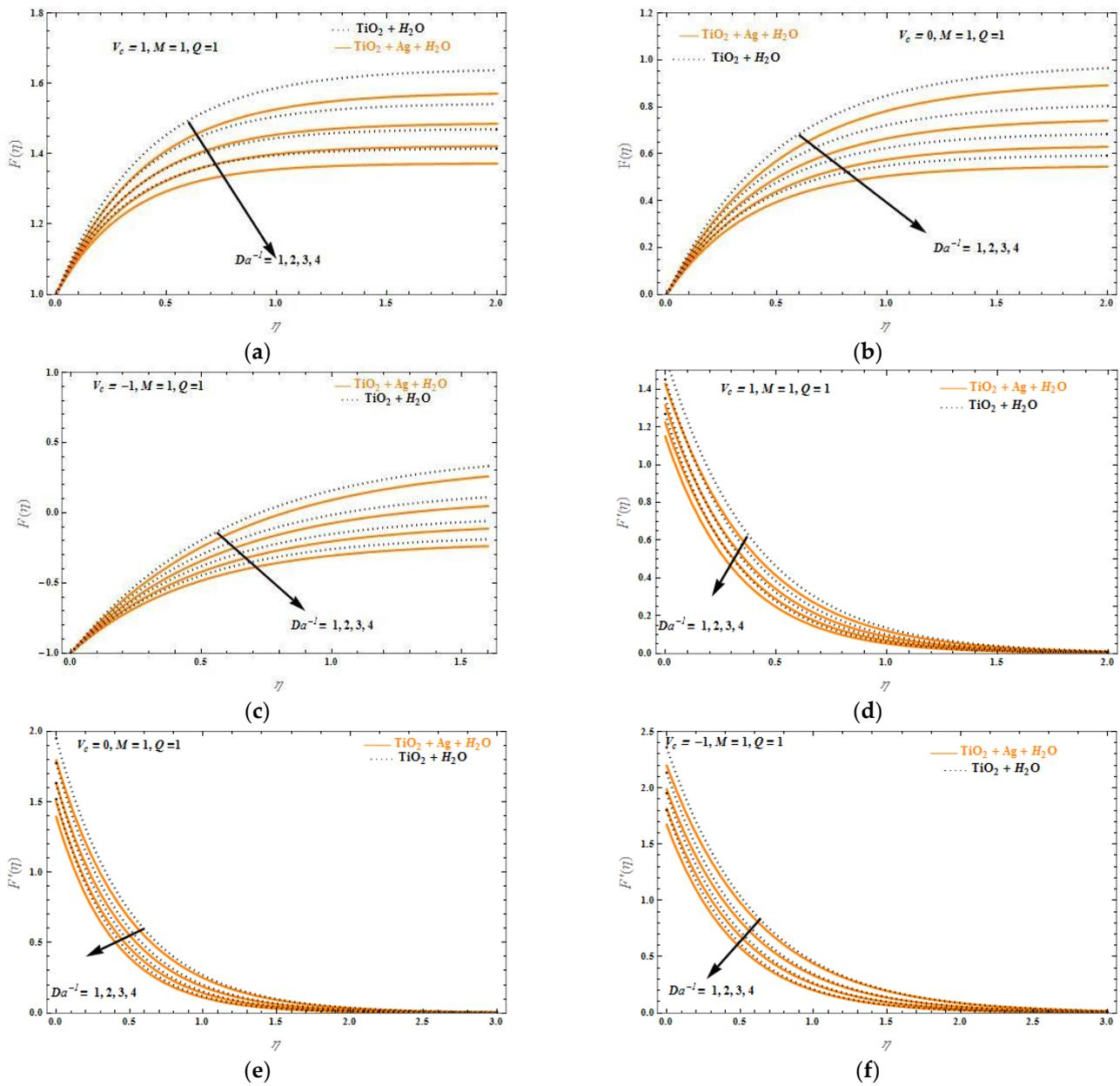
**Figure 4.** The axial,  $F(\eta)$ , and transverse,  $F'(\eta)$ , velocities versus the similarity variable,  $\eta$ , for various values of  $Da^{-1}$  and  $Q = M = 1$ . (a)  $F(\eta)$ , for  $V_c = 1$ , (b)  $F(\eta)$ , for  $V_c = 0$ , (c)  $F(\eta)$ , for  $V_c = -1$ , (d)  $F'(\eta)$ , for  $V_c = 1$ , (e)  $F'(\eta)$ , for  $V_c = 0$ , and (f)  $F'(\eta)$ , for  $V_c = -1$ . The orange solid line refers to the  $(TiO_2-Ag, H_2O)$  HNF and dotted line to  $(TiO_2, H_2O)$ .
