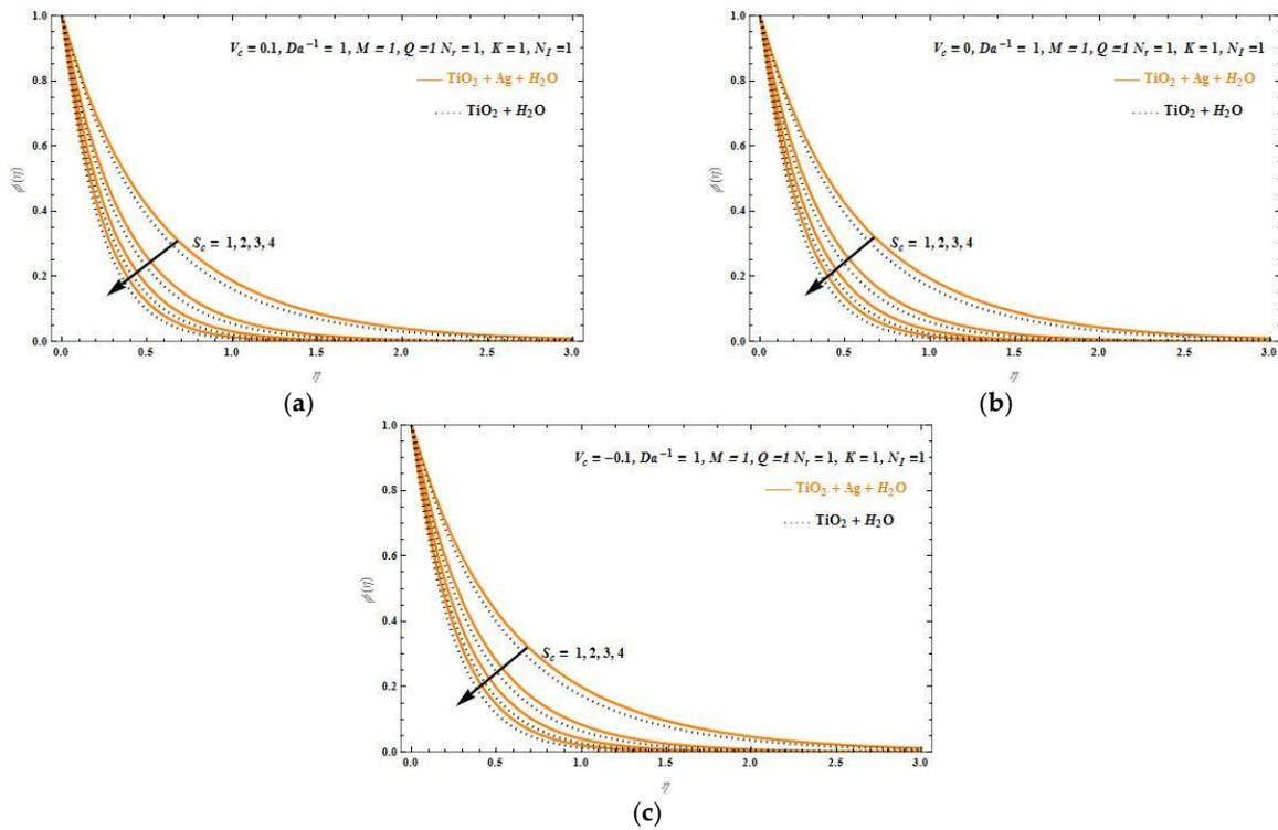
Figure 14. Concentration profiles,  $\phi(\eta)$ , versus similarity variable,  $\eta$ , for various Schmidt number,  $S_c$ , values,  $Da^{-1} = N_I = N_r = M = Q = K = 1$ , and (a)  $V_c = 0.1$ , (b)  $V_c = 0$ , and (c)  $V_c = -0.1$ .
