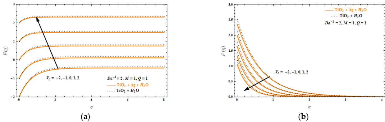
**Figure 8.** (a) Axial,  $F(\eta)$ , and (b) transverse,  $F'(\eta)$ , velocities versus the similarity variable,  $\eta$ .  $M = Q = 1$ ,  $Da^{-1} = 2$ . The orange solid line refers to the  $(TiO_2-Ag, H_2O)$  HNF and dotted line to  $(TiO_2, H_2O)$ .
