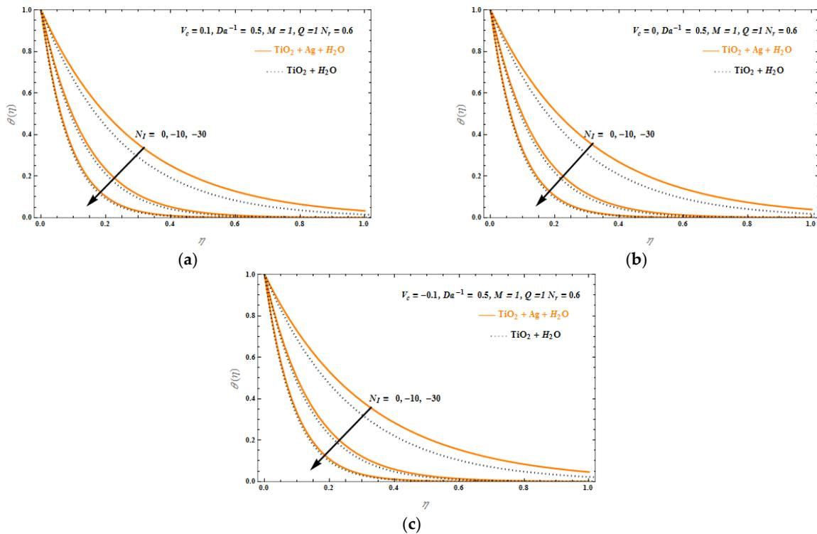
**Figure 10.** Temperature profiles,  $\theta(\eta)$ , versus similarity variable,  $\eta$ , for various heat source and sink parameter,  $N_I$ , values,  $Da^{-1} = 0.5$ ,  $N_r = 0.6$ , and  $M = Q = 1$ , and (a)  $V_c = 0.1$ , (b)  $V_c = 0$ , and (c)  $V_c = -0.1$ .
