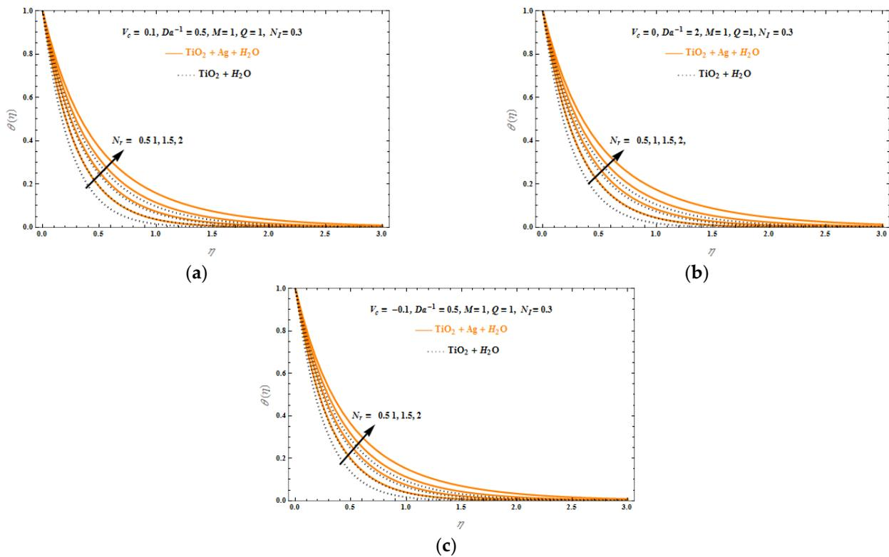
**Figure 9.** Temperature profiles,  $\theta(\eta)$ , versus similarity variable,  $\eta$ , for various thermal radiation parameter,  $N_r$ , values,  $Da^{-1} = 0.5$ ,  $N_l = 0.3$ , and  $M = Q = 1$ , and (a)  $V_c = 0.1$ , (b)  $V_c = 0$ , and (c)  $V_c = -0.1$ .
