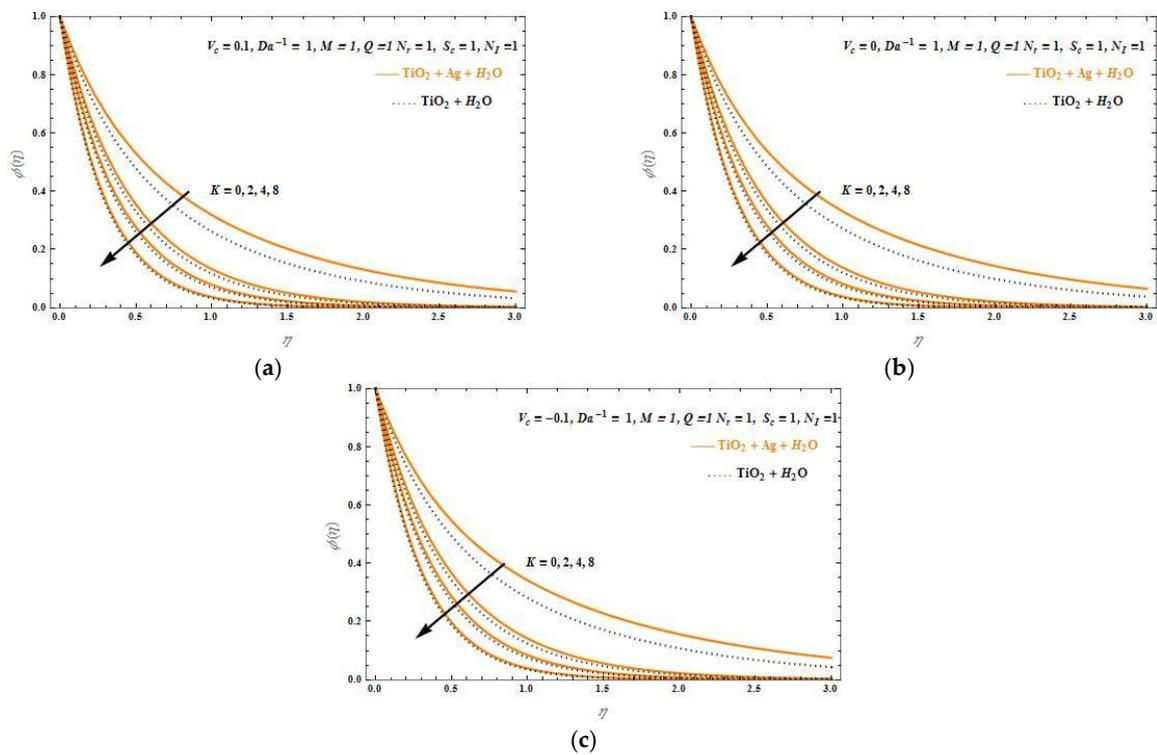
**Figure 13.** Concentration profiles,  $\phi(\eta)$ , versus similarity variable,  $\eta$ , for various chemical reaction coefficient,  $K$ , values,  $Da^{-1} = N_l = N_r = M = Q = S_c = 1$ , and (a)  $V_c = 0.1$ , (b)  $V_c = 0$ , and (c)  $V_c = -0.1$ .
