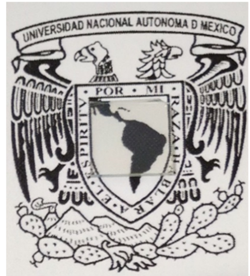
Figure 4. (a) Tauc scattering of direct transitions for ZnO:Al deposited on fused silica substrate (squares) and glass substrate (circles). Linear fit extrapolation was taken over a range of 3.4 to 4 eV in both cases and is presented by a red dotted line. See text for details. (b) Photograph of ZnO:Al film deposited on glass substrate showing exceptionally good homogeneity at the macroscopic level.
