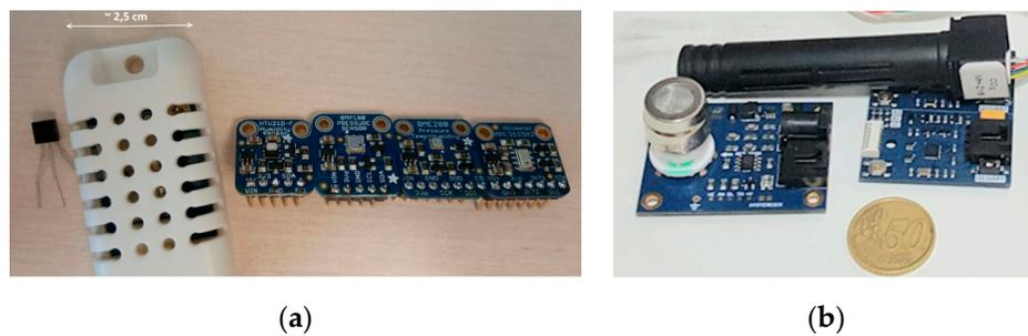
**Figure 1.** (a) Climatic sensors used in this study. From left to right: DS18B20, AM2302, HTU21D, BMP180, BME280 and MPL3115A2. (b) Carbon dioxide sensors used in this study. From left to right: MG-811 and MH-Z16.
