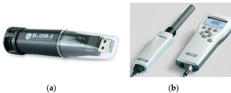
**Figure 2.** Reference instruments used in this study for (a) temperature and humidity and (b) carbon dioxide.
