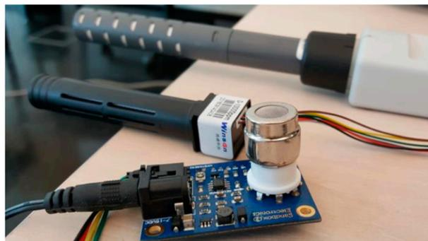
**Figure 4.** A single unit of each carbon dioxide sensor placed in the office room (MG-811 sensor in the bottom of the image and MH-Z16 sensor in the middle), and the reference sensor (in the top of the image) for calibration purposes.
