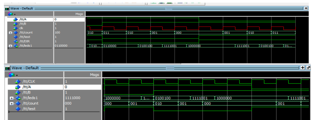
Figure 12. Hardware Trojan Simulation in ModelSim.
